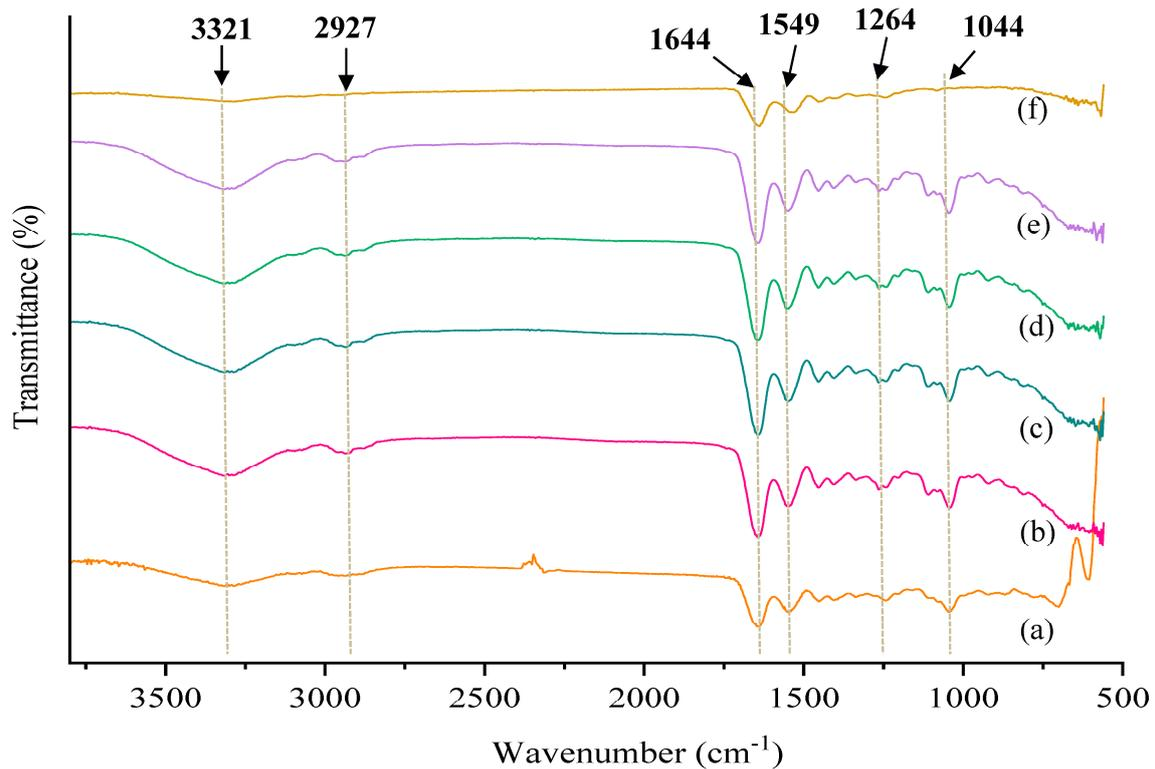
**Figure 2.** FTIR–ATR spectra of transglutaminase (TGase) cross-linked tilapia collagen (TC) films incorporated with lysozyme (LYS). (a) TC-TGase-LYS-0, (b) TC-TGase-LYS-2, (c) TC-TGase-LYS-4, (d) TC-TGase-LYS-6, (e) TC-TGase-LYS-8 and (f) Lysozyme.
