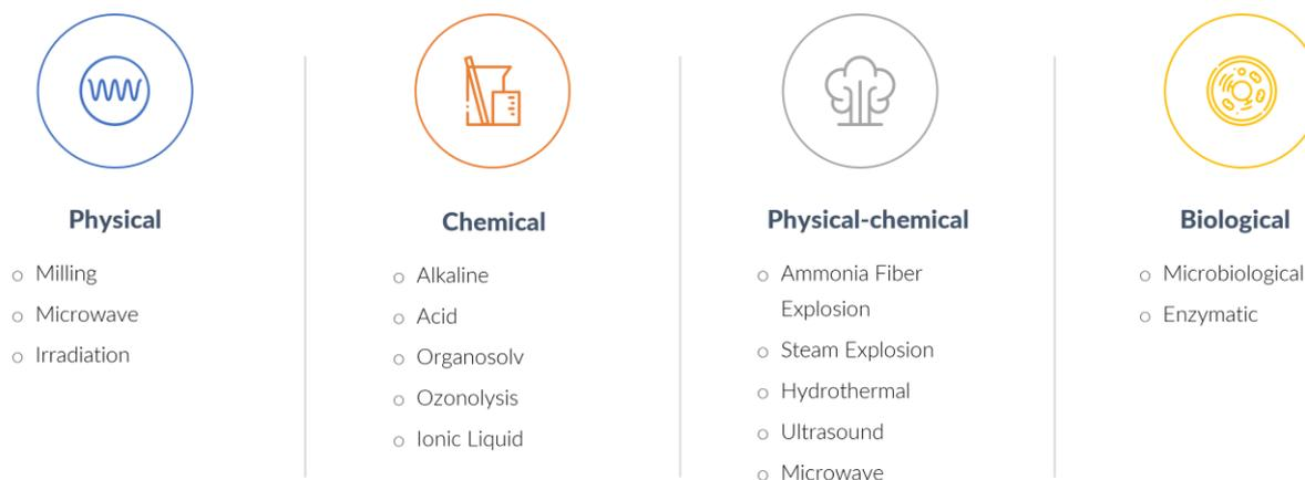
Figure 6. Biomass pretreatments methods (adapted from Aguiar et al. [23]).
