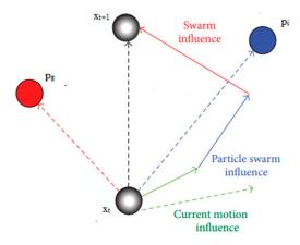
Figure 2. Illustration of particle's position after being subjected to PSO.
