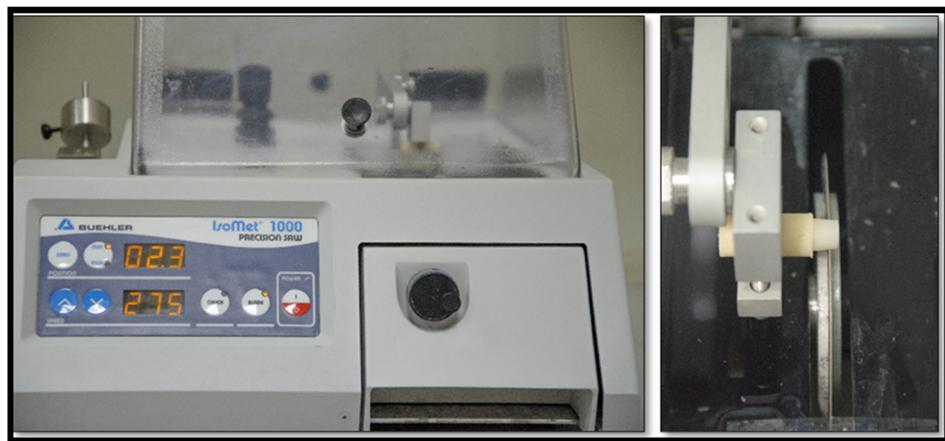
**Figure 8.** Cutting the sample into two slices with a thickness of 2 mm each.
