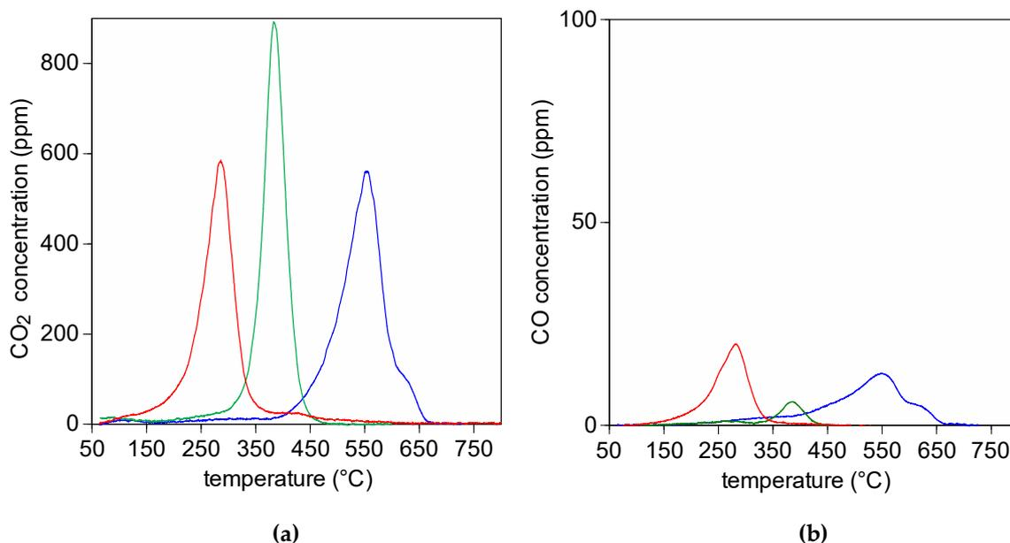
**Figure 3.** Temperature programmed oxidation (TPO) profiles of (a) CO<sub>2</sub> and (b) CO evolved from CZ/C mixtures at different mixing condition: CZ(l) (blue), CZ(t) (green) and CZ(m) (red).
