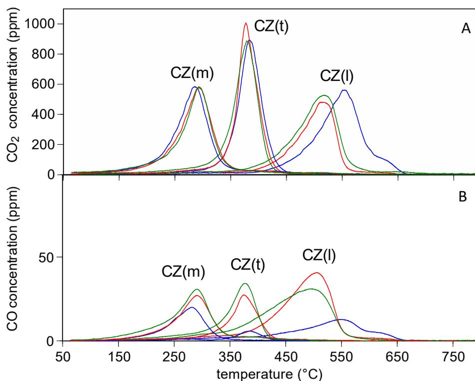
**Figure 4.** (A)  $CO_2$  evolution and (B)  $CO$  evolution from temperature programmed oxidation (TPO) profiles for CZ/C mixtures at different mixing condition and different atmosphere:  $O_2$  (blue),  $NO+O_2$  (red) and  $NO_2+O_2$  (green).
