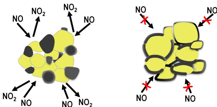
**Figure 6.** Scheme of  $\text{NO}_x$  interaction over CZ(t) and CZ(l) (left) and CZ(m) (right). Ceria–zirconia particles are indicated in yellow, while carbon agglomerates and carbon layers are indicated in black.
