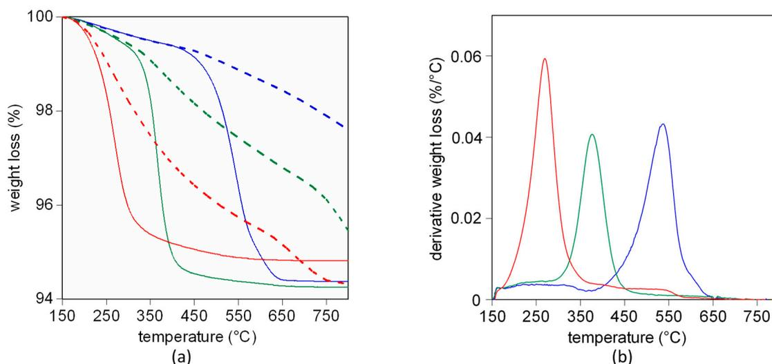
**Figure 2.** (a) Weight loss profile analysis of CZ/carbon mixtures in air (solid line) and in  $N_2$  (dashed line) under different contact conditions and (b) derivative weight loss profile in air: CZ(l) (blue), CZ(t) (green) and CZ(m) (red).
