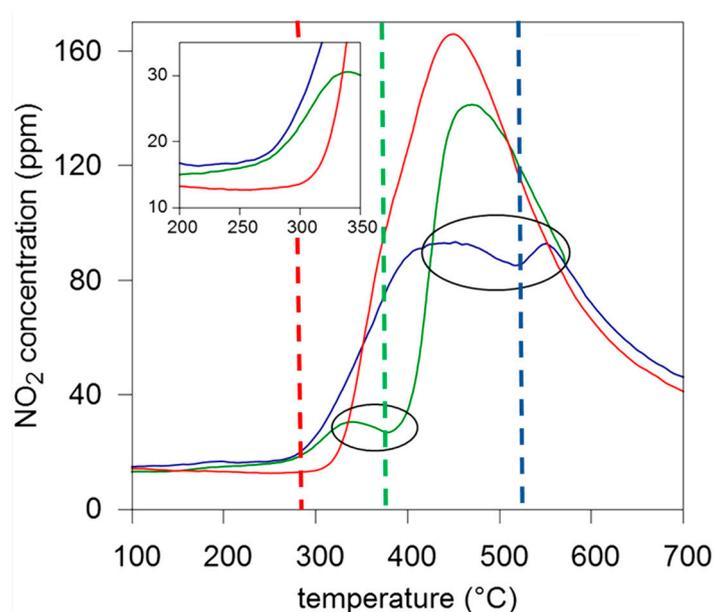
**Figure 5.** Temperature programmed oxidation (TPO) profiles of  $\text{NO}_2$  evolved from CZ/C mixtures at different mixing condition under  $\text{NO}+\text{O}_2$  gas flow: CZ(l) (blue), CZ(t) (green) and CZ(m) (red). Dotted lines indicate  $T_p$  of carbon oxidation (from red line in Figure 4).
