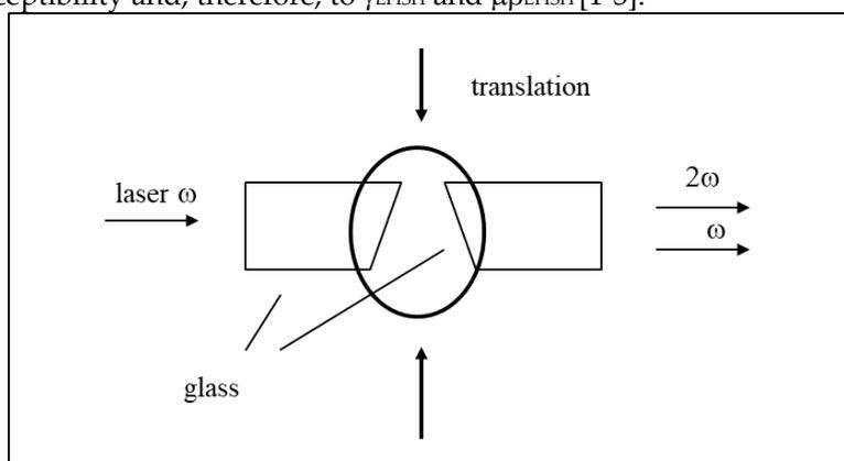
Figure S2. Top view of the EFISH cell.
