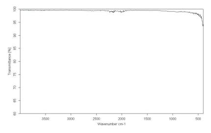
Figure S1: IR spectrum of RbF and Rb<sub>2</sub>S measured on an ATR diamond module.
