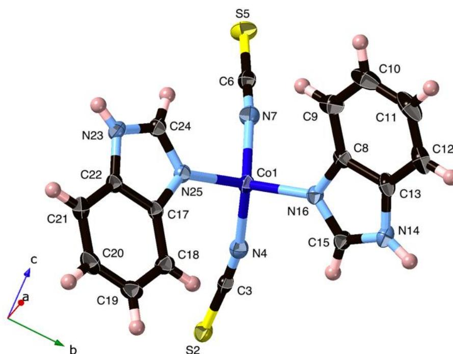
**Figure 2.** Molecular structure of the new polymorph  $\gamma$ - $[\text{Co}(\text{Hbzim})_2(\text{SCN})_2]$  from single-crystal X-ray diffraction. Displacement ellipsoids drawn at 50%. Note the conformation of the two benzimidazole ligands arranged with benzene rings on opposite sides.
