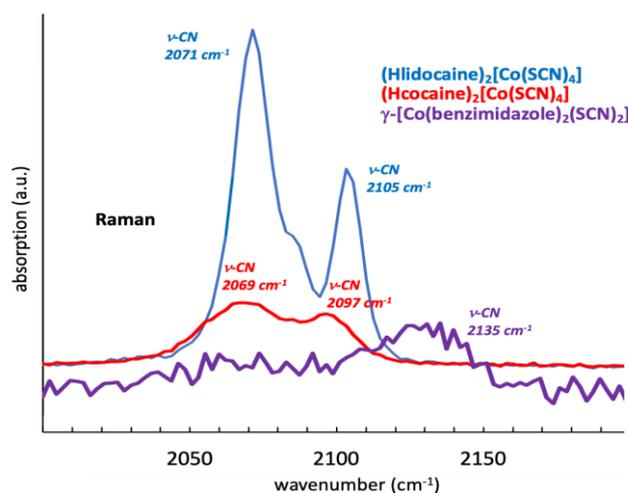
**Figure 4.** The distinctive Raman bands around  $2100\text{ cm}^{-1}$  for blue precipitates retrieved from representative cocaine hydrochloride (—), lidocaine monohydrate hydrochloride (—), and benzimidazole (—) reaction vessels. Usually, these bands are interpreted as  $\text{C}\equiv\text{N}$  stretching.
