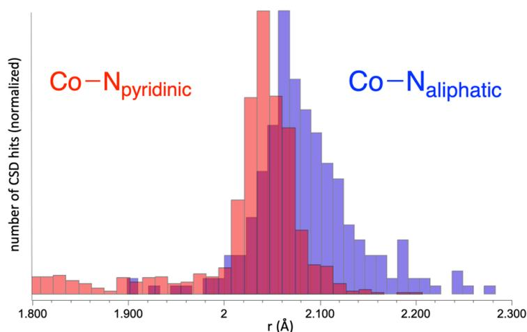
**Figure 6.** Comparison of four-coordinated Co(II) structures with at least one coordinated pyridine unit (representing aromatic amines; total number of hits: 614) to four-coordinated Co(II) structures with a Co-N bond and a nitrogen with three single bonds to either carbon or hydrogen (total number of hits: 168). The aromatic compounds have a most probable Co-N distance of 2.04 Å and the aliphatic amines a most probable Co-N distance of 2.06 Å.
