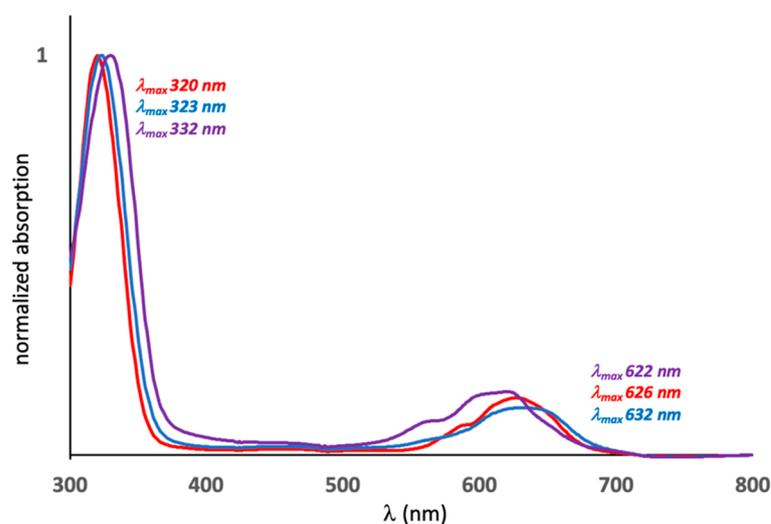
**Figure 3.** UV-vis spectra in ethyl acetate solution of blue precipitates from cocaine hydrochloride (—), lidocaine monohydrate hydrochloride (—), and benzimidazole (—) reaction products with cobalt thiocyanate.
