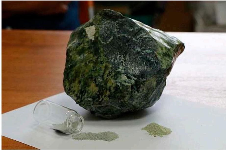
Figure 2. Natural serpentinite ore and grinding powders.
