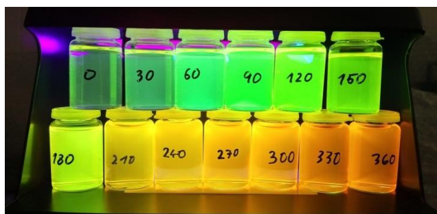
Figure S9: The picture of samples of CdTe-QD nanoparticles covered by MPA. The samples were taken in the course of heating of mixture under reflux.
