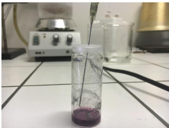
Figure S2: The first step of synthesis of NaHTe used for preparation of CdTe.
