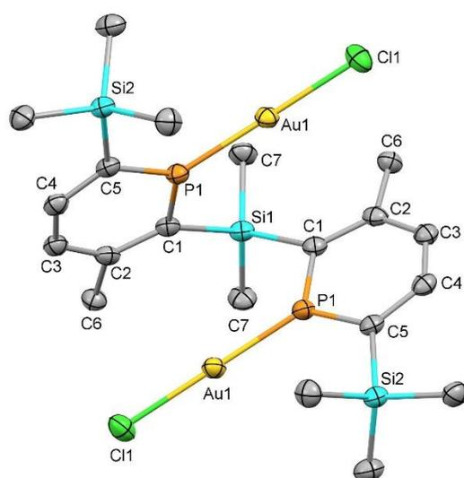
**Figure 2.** Molecular structure of **21** (thermal ellipsoids at 50%; all H atoms have been omitted for clarity). Selected bond lengths (Å) and angles ( $^\circ$ ): Au1-Cl1 2.2742(12), Au1-P1 2.2078(12), P1-C1 1.721(4), P1-C5 1.709(4), C1-C2 1.396(6), C2-C3 1.398(6), C2-C6 1.524(6), C3-C4 1.396(6), C4-C5 1.388(6), P1-Au1-Cl1 178.13(4),  $\eta^2$  interaction: Au1-C1' 3.287, Au1-C2' 3.460.
