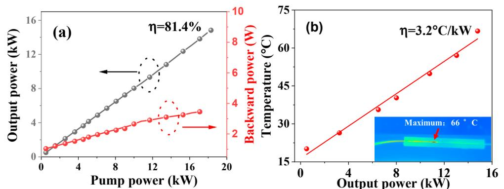
**Figure 8.** (a) The output power and efficiency results of the amplifier; (b) the temperature results of the amplifier.
