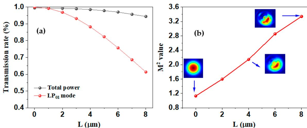
**Figure 2.** Theoretical relationships between the core off-axis value with the signal transmission rate (a) and the  $M^2$  value (b).
