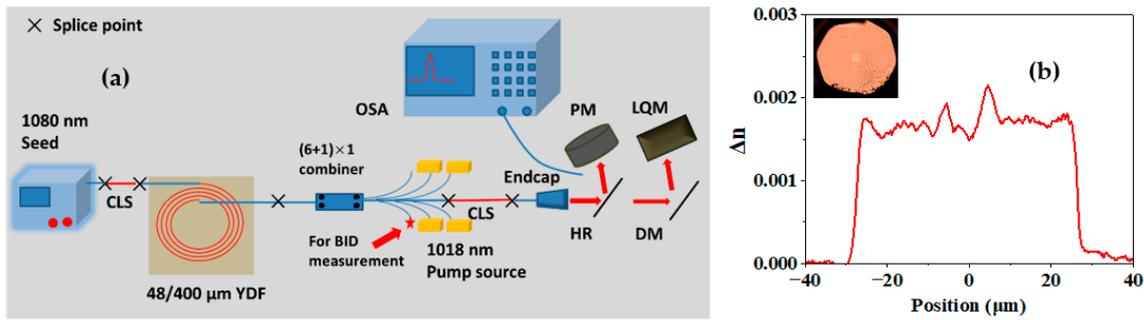
**Figure 7.** (a) Experimental setup of the counter-directional tandem-pumping fiber amplifier based on the home-made pump-signal combiner: CLS, cladding light stripper; HR, highly reflective mirror; DM, dichroic mirror; PM, power meter; OSA, optical spectrum analyzer; LQM, beam quality analyzer. (b) The measured refractive index profile of the gain fiber.
