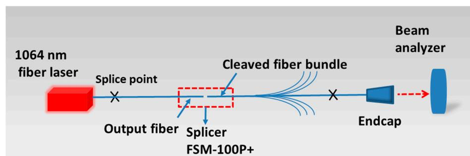
**Figure 4.**  $M^2$ -based in-line alignment splicing structure.
