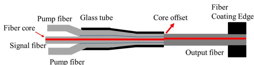
**Figure 1.** The brief diagram of the pump-signal combiner.
