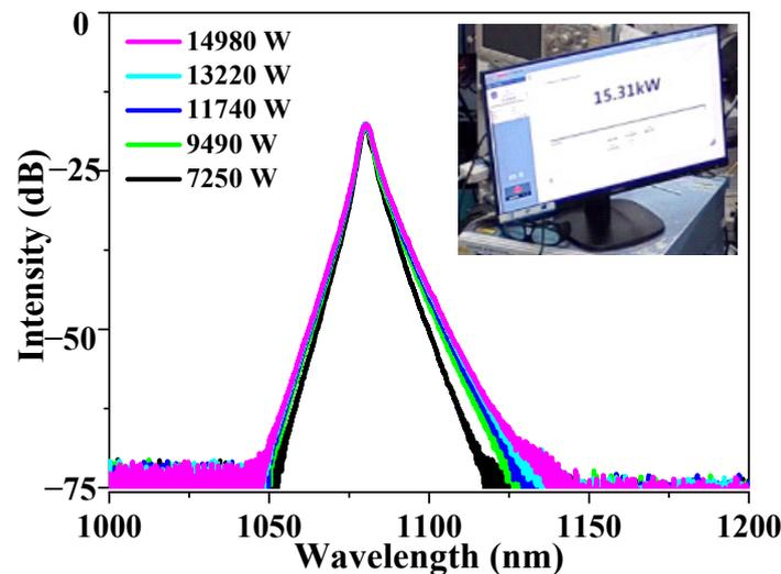
**Figure 9.** The spectrum of the amplifier at different output power.
