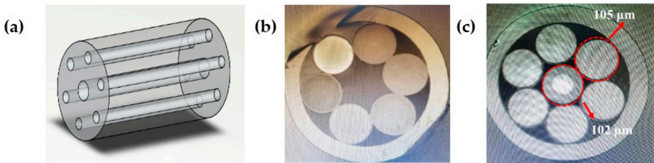
**Figure 3.** (a) The structure diagram of the seven-hole glass tube; microscopic images of the TFB before (b) and after (c) the central fiber inserted.
