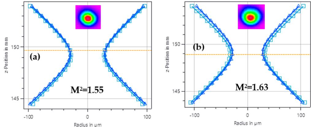
Figure 6. The  $M^2$  value of the signal light before (a) and after (b) transmitting the home-made combiner.
