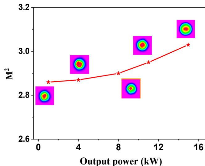
Figure 10. The  $M^2$  value of the amplifier at different output power.
