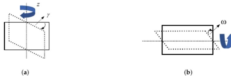
Figure 2. (a) The mirror’s yaw rotation angle. (b) The mirror’s roll rotation angle.
