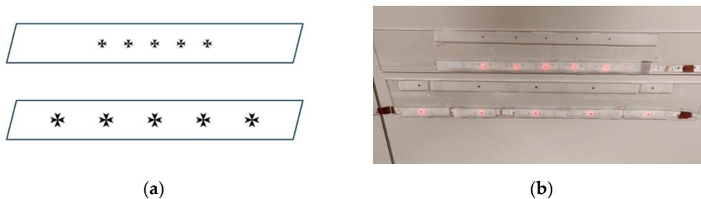
**Figure 2.** Methacrylate accessory plates: (a) Superior plate presenting the stimuli for 5 D of accommodative demand and inferior plate presenting the stimuli for 2.5 D of accommodative demand; (b) Final accessory plates with an identical second set of red LED backlit stimuli for each accommodative distance.
