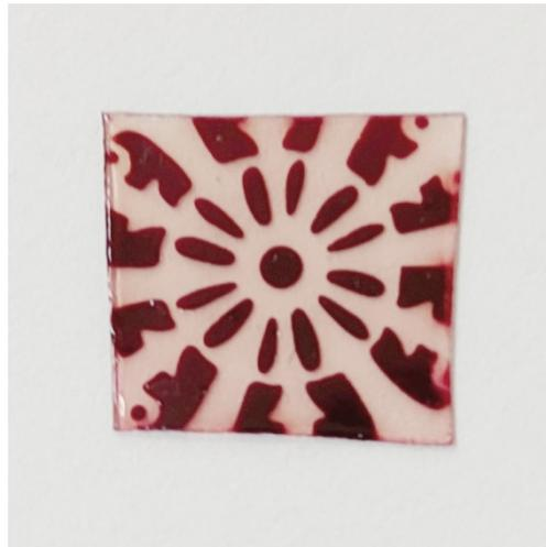
**Figure 5.** The sample after irradiation through the mask and further heating.
