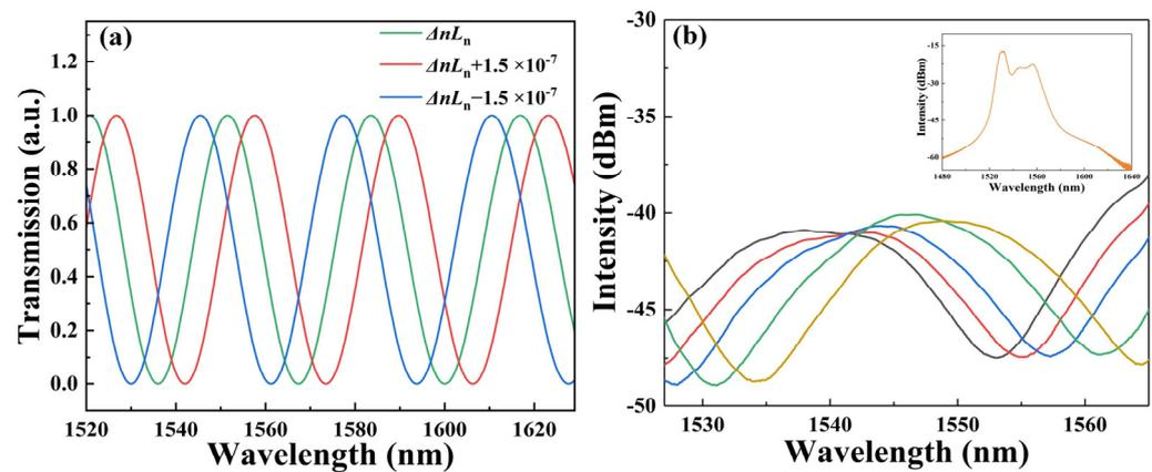
**Figure 2.** (a) Filtering curves under stress birefringence effects. (b) Experimentally measured filtering spectrum (inset: the amplified spontaneous emission of EDF).
