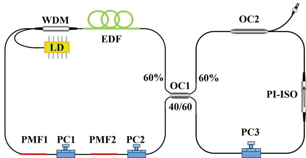
**Figure 1.** Schematic diagram of wavelength-tunable fiber laser based on NALM mode-locking. LD: laser diode; WDM: wavelength division multiplexer; EDF: er-doped fiber; PC: polarization controller; PMF: polarization-maintaining fiber; OC: optical coupler; PI-ISO: polarization-independent optical isolator.
