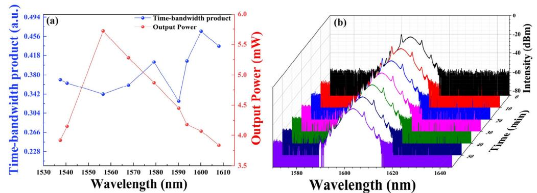
**Figure 5.** (a) Time-bandwidth product and output power versus wavelength; (b) Spectral stability.
