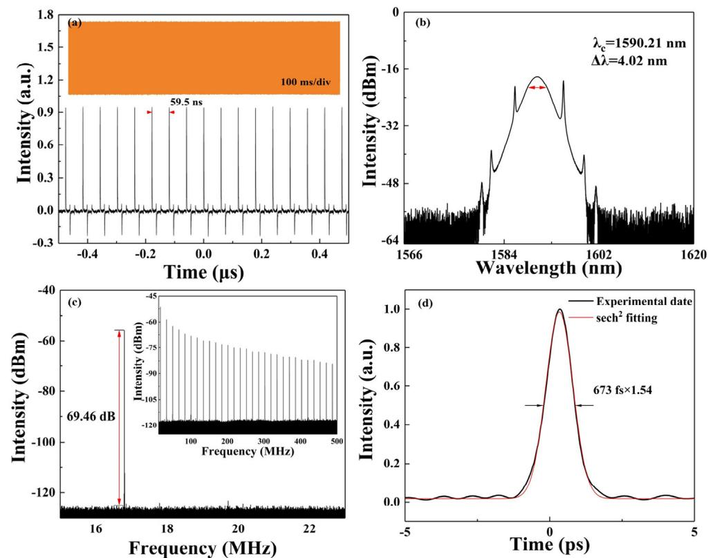
**Figure 3.** Typical mode-locked characteristics at 200 mW pump power. (a) Oscilloscope pulse traces; (b) Spectrum of the output pulses; (c) RF spectrum (inset: broadband RF spectrum in 500 MHz range); (d) Corresponding autocorrelation trace.
