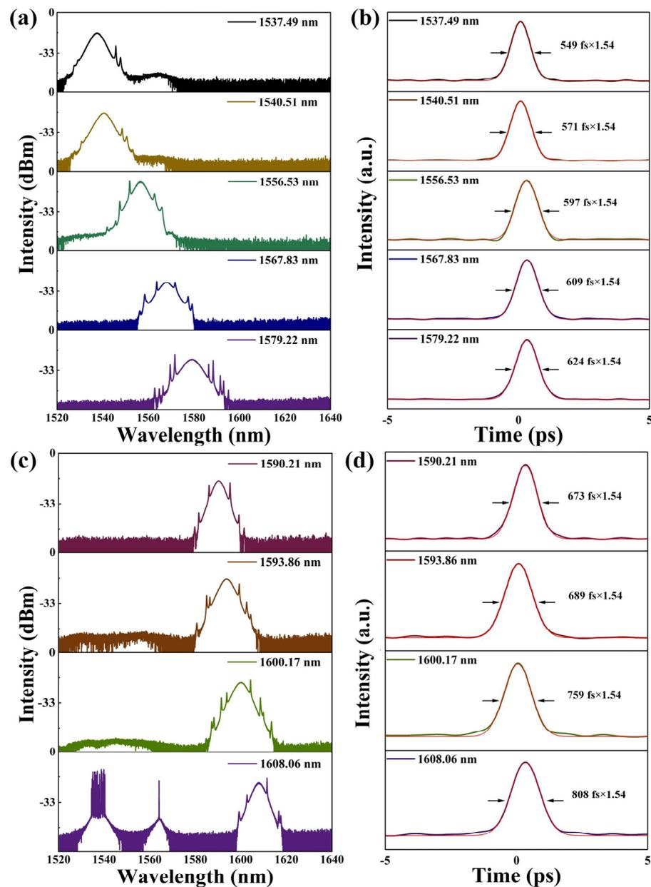
**Figure 4.** On the left, (a,c) are spectrum with tunable wavelength; the right columns (b,d) are the corresponding pulse widths collected by the autocorrelator.
