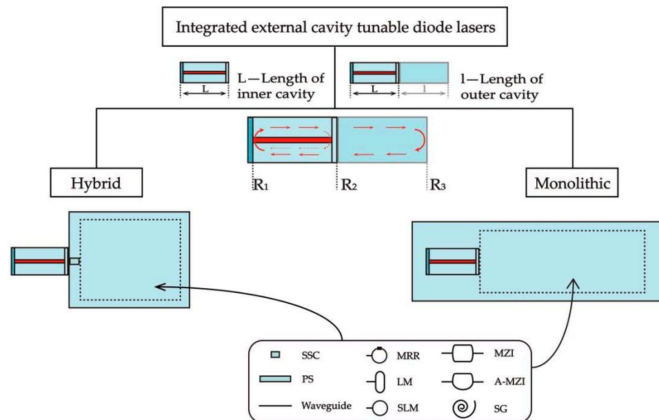
**Figure 1.** Basic structure of an integrated external cavity tunable diode laser. Note: gain chip (GC), spot size converter (SSC), phase shifter (PS), micro-ring resonator (MRR), loop mirror (LM), Sagnac loop mirror (SLM), Mach–Zehndel interferometer (MZI), asymmetry Mach–Zehndel interferometer (A-MZI), and spiral grating (SG).
