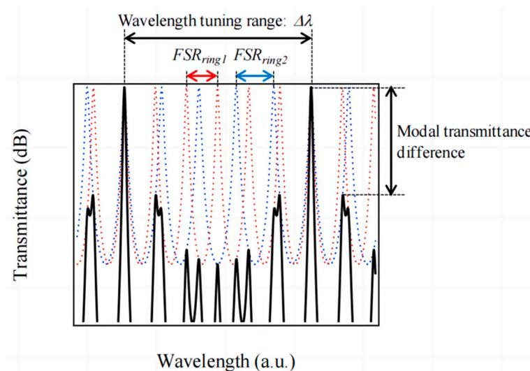
**Figure 4.** Wavelength tunable principle of monolithic integrated external cavity tunable diode laser. The red dashed line is transmittance of the  $FSR_{ring1}$  and the blue dashed line is the transmittance of the  $FSR_{ring2}$  and the black solid line is the total transmittance.
