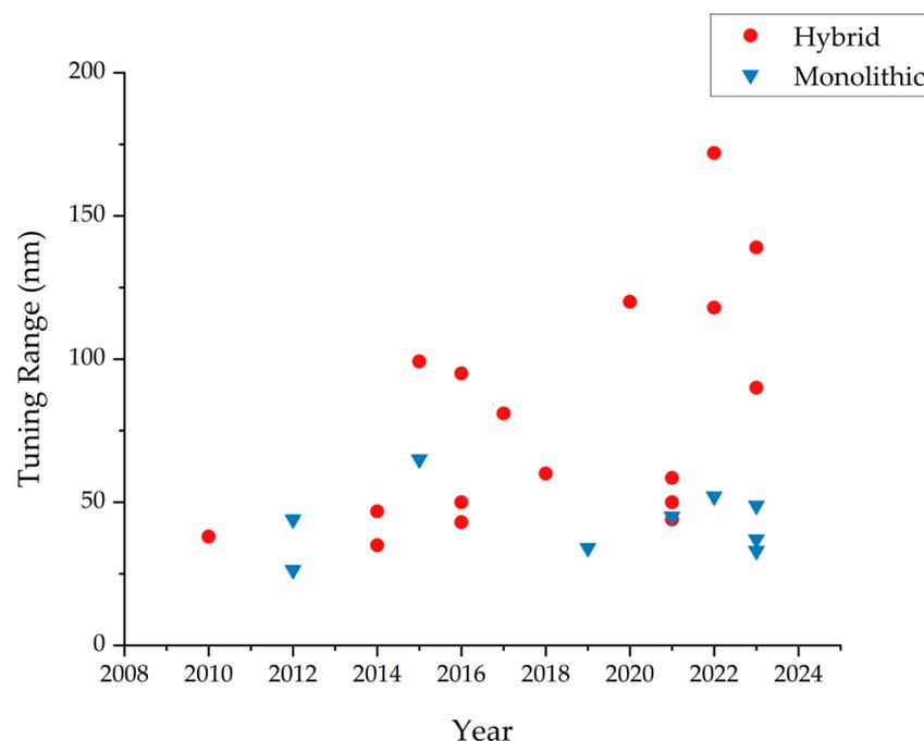
**Figure 5.** Comparison of the tuning range of 1.55  $\mu\text{m}$  waveband hybrid integrated and monolithic integrated external cavity tunable diode lasers.
