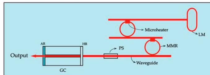
Figure 3. Monolithic integrated external cavity tunable diode laser.
