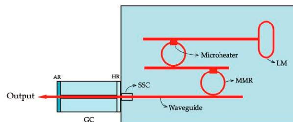
**Figure 2.** The structure of hybrid integrated external cavity tunable diode lasers.
