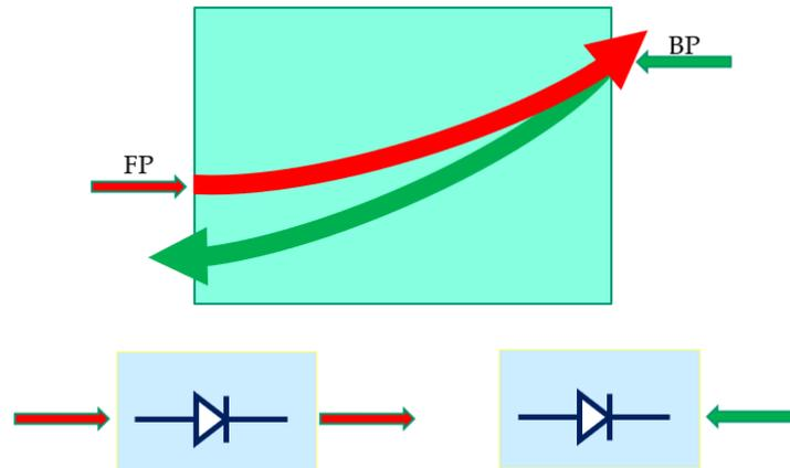
**Figure 1.** Artistic rendering of a nematicon-based optical diode. The FP soliton and associated waveguide do not overlap with the BP soliton and associated waveguide, effectively isolating the FP input port from the BP light. The FP nematicon and signal are transmitted (red arrows), left bottom panel, the BP nematicon and signal are not transmitted through the FP input port, right bottom panel.
