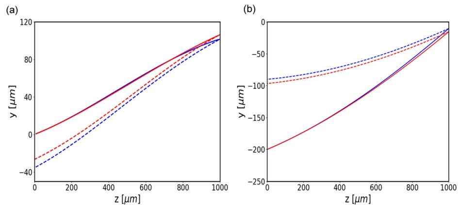
**Figure 6.** Comparison of nematicon trajectories for FP (solid lines) and BP (dashed lines) beams in the lossless limit (blue lines) and in the presence of typical propagation losses of  $5\text{ cm}^{-1}$  (red lines): (a) linear longitudinal modulation from  $\theta_0 = 15^\circ$  to  $\theta_L = 55^\circ$ ; (b) linear transverse modulation from  $\theta_{bot} = 30^\circ$  to  $\theta_{top} = 50^\circ$ .
