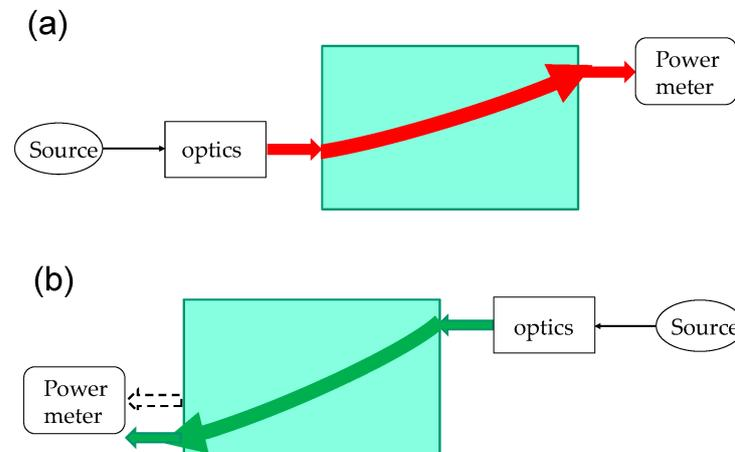
**Figure 7.** Isolator operation: (a) FP nematicon and guided-wave copolarized signal travel from left to right, reaching the light meter; (b) BP nematicon and copolarized guided signal travel from right to left using the same FP output port, but do not reach the detector, as they follow the green path despite the identical beam excitation with  $k_{FP} = -k_{BP}$ .
