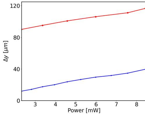
**Figure 4.** Beam power dependence of transverse separation  $\Delta y$  for linear longitudinal modulation (blue line with calculated data points) and linear transverse modulation (red line with calculated datapoints) in the same intervals of  $\theta$  as in Figure 3 above and Figure 5 below, respectively.
