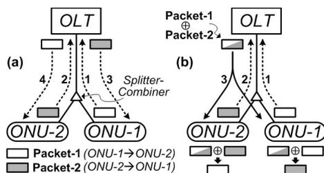
Figure 4. Performance enhancements of an EPON through network coding.
