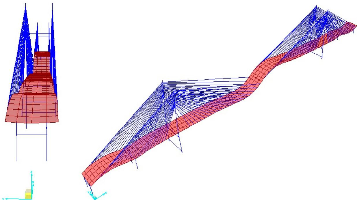
**Figure 17.** Antisymmetric bending mode shape of the FRP cable-stayed bridge (0.4009 Hz).
