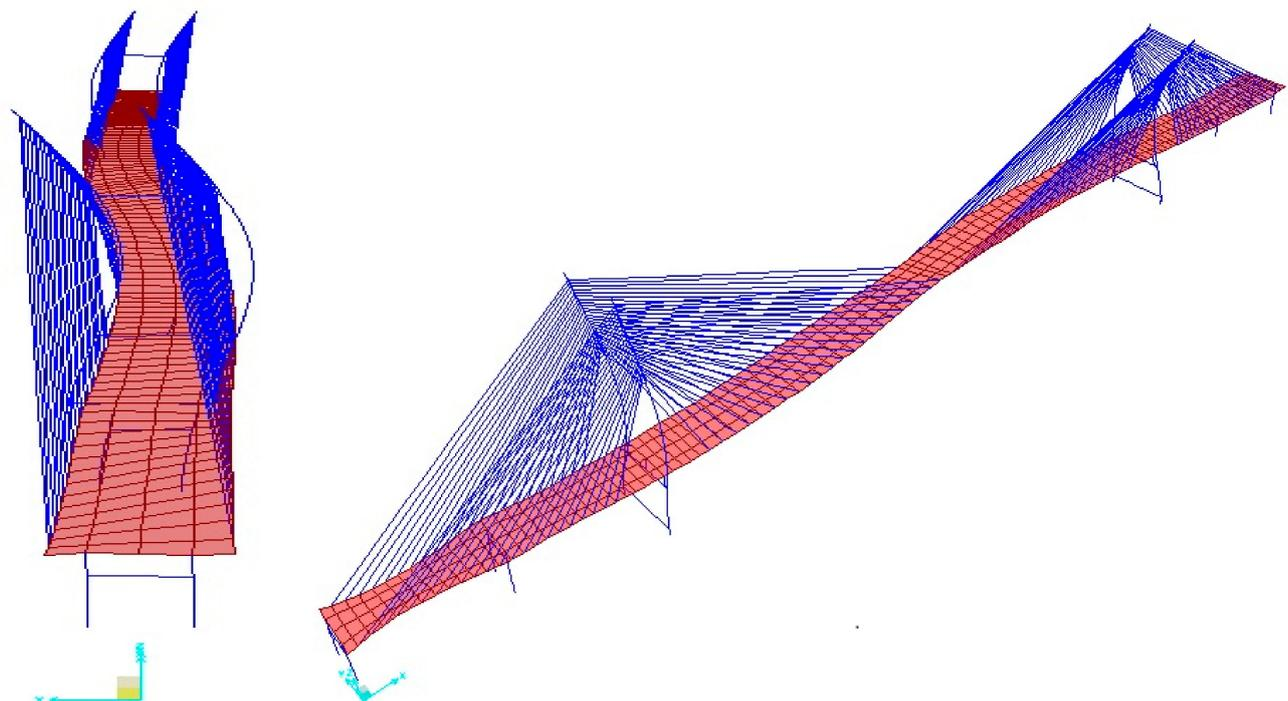
**Figure 11.** Antisymmetric lateral mode shape of the FRP cable-stayed bridge (1.003 Hz).
