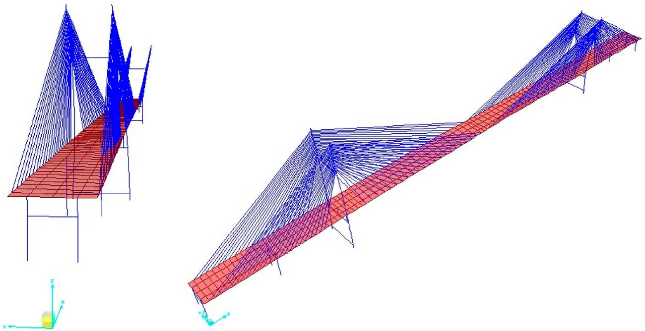
**Figure 15.** Antisymmetric tower dominant mode shape of the FRP cable-stayed bridge (0.2245 Hz).
