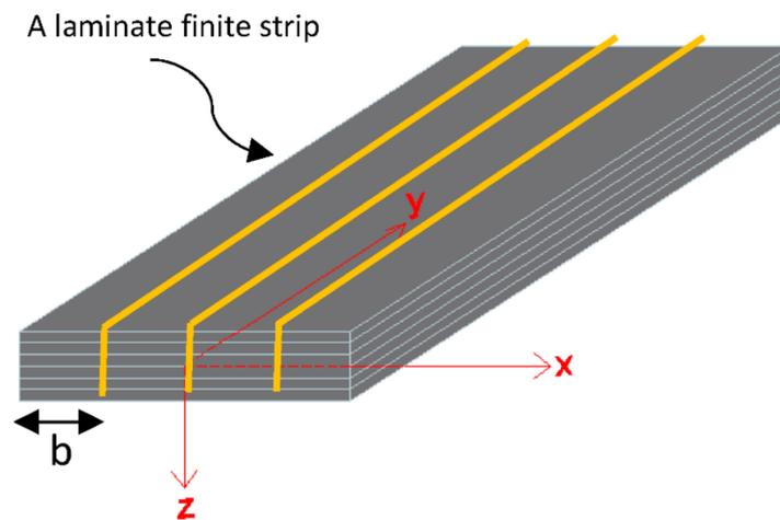
Figure 1. Multi-layer composite plate divided by laminate finite strips.
