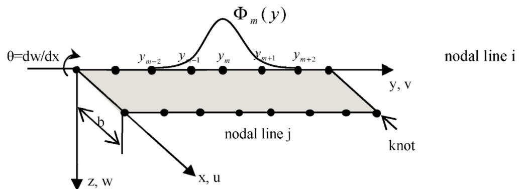
Figure 2. Laminate spline finite strip.
