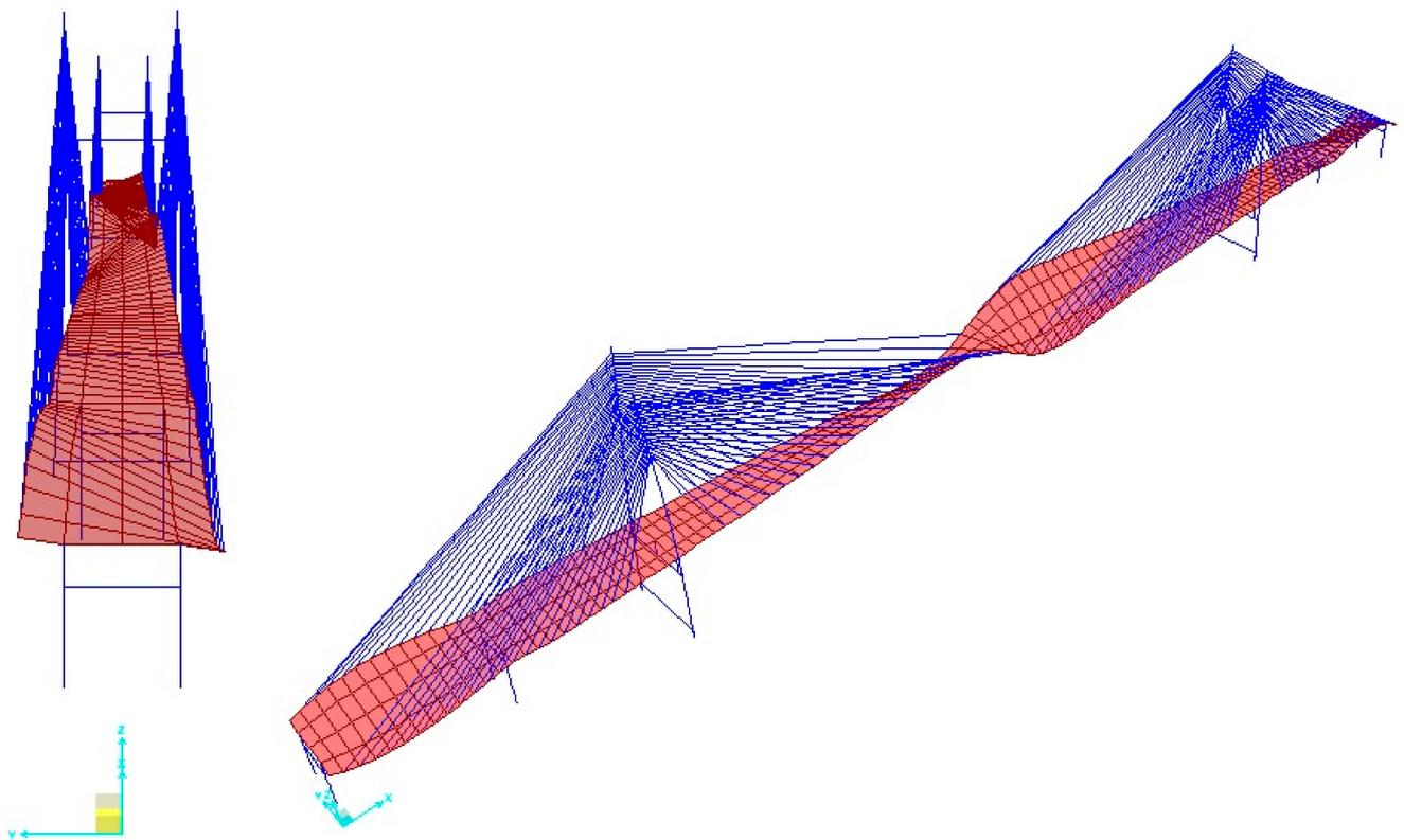
Figure 13. Antisymmetric torsional mode shape of the FRP cable-stayed bridge (0.6290 Hz).
