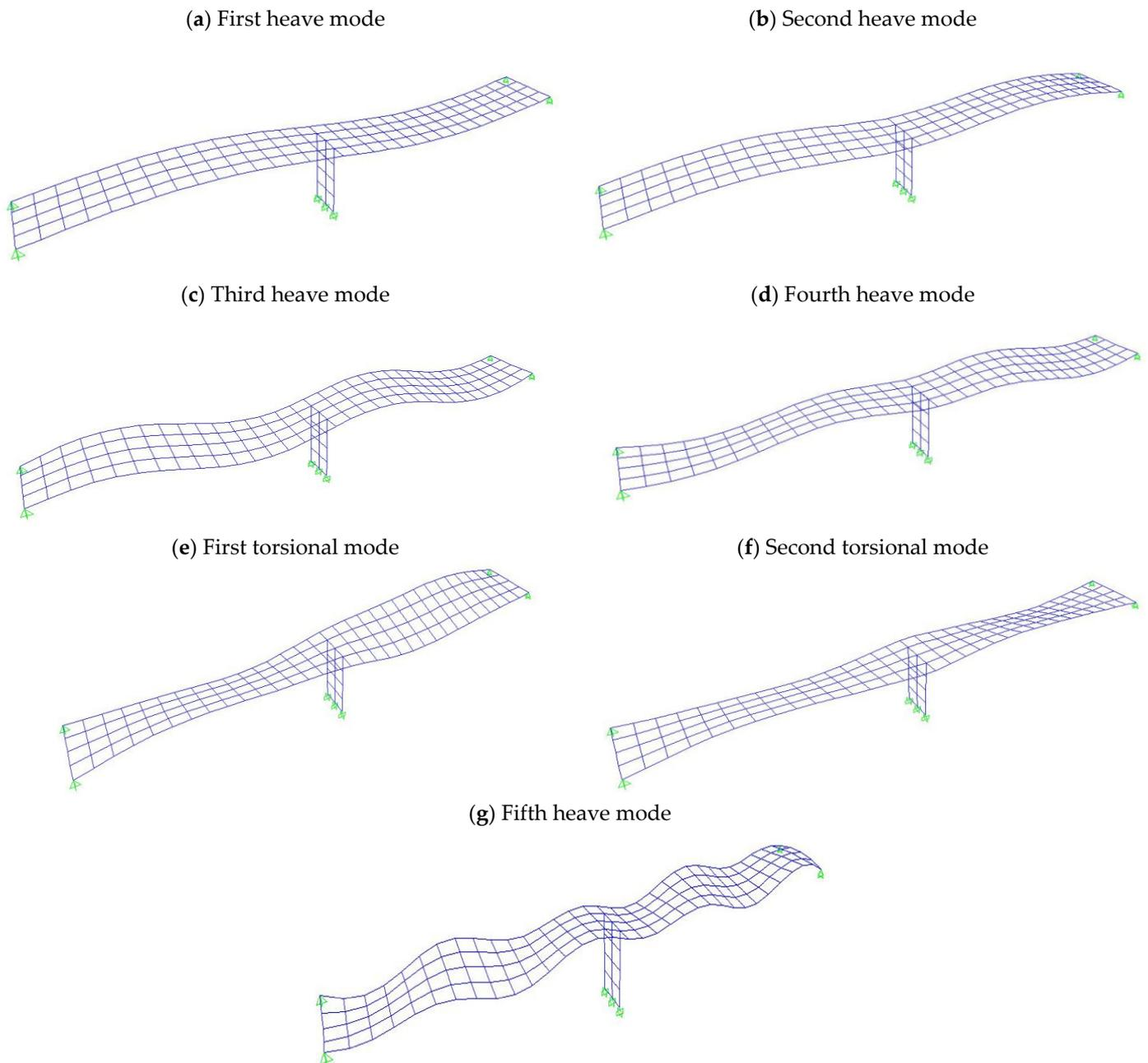
**Figure 7.** Mode shapes of the FRP deck bridge.
