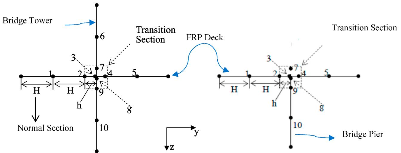
Figure 5. Typical transition section elements for tower (left) and pier (right).
