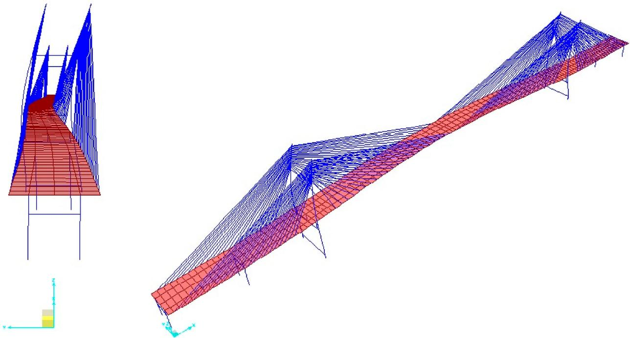
**Figure 10.** Symmetric lateral mode shape of the FRP cable-stayed bridge (0.5725 Hz).
