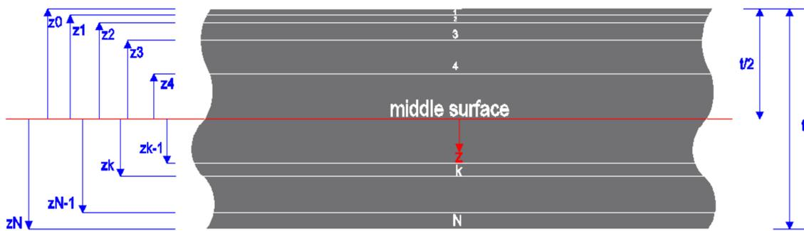
Figure 4. Laminated plate cross-sectional geometry and ply numbering system.
