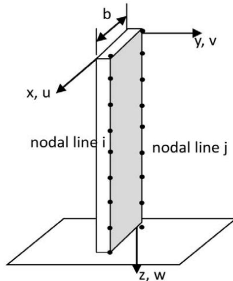
Figure 3. Column strip in local coordinate system (CS).
