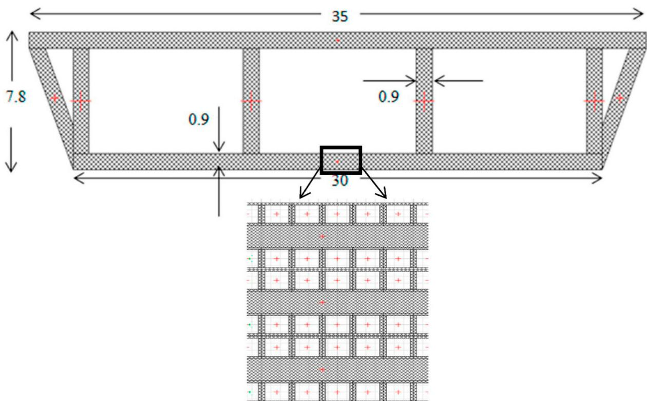
**Figure 9.** Design of the FRP bridge deck system (dimensions are in meters) [25].
