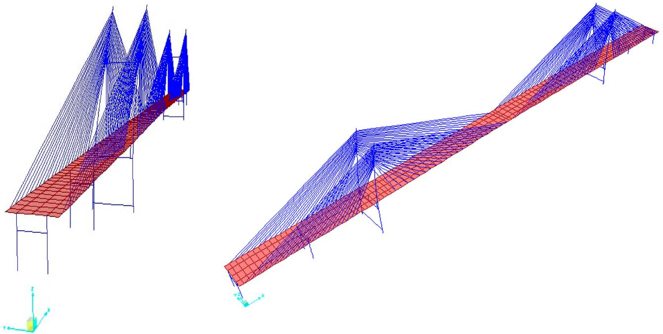
**Figure 14.** Symmetric tower dominant mode shape of the FRP cable-stayed bridge (0.1986 Hz).
