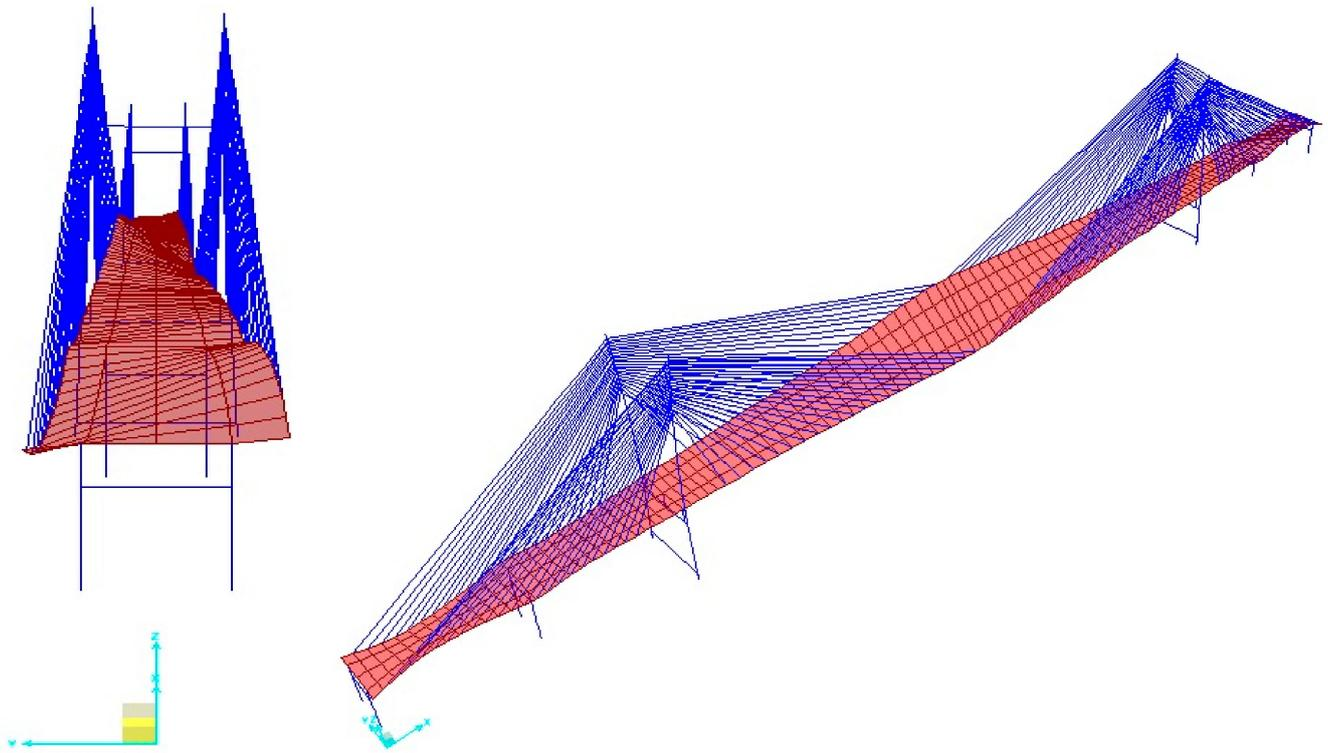
Figure 12. Symmetric torsional mode shape of the FRP cable-stayed bridge (0.5027 Hz).
