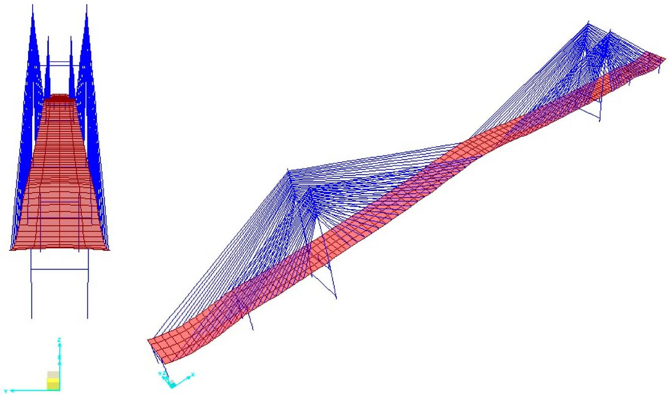
**Figure 16.** Symmetric bending mode shape of the FRP cable-stayed bridge (0.3354 Hz).
