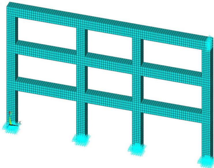
**Figure 3.** The FE mesh of the R/C frame model
