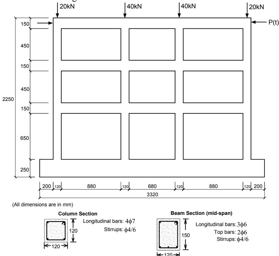
**Figure 2.** The geometry, cross-sections and rebar details of the R/C frame
