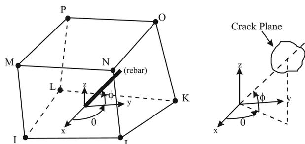
**Figure 1.** *Solid65* element type as defined in ANSYS
