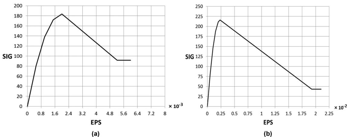
**Figure 6.** The  $\epsilon$ - $\sigma$  relationship of *Multilinear Isotropic Hardening Model* for: (a) Unconfined concrete (b) Confined concrete (SIG: kg/cm<sup>2</sup>)
