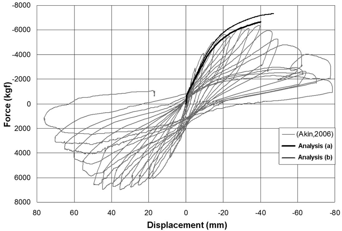
**Figure 7.** Comparison of analyses results under monotonic loading with the experimental data
