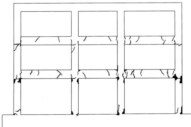
**Figure 13.** Observed crack profile at the maximum displacement by Akin [13]
