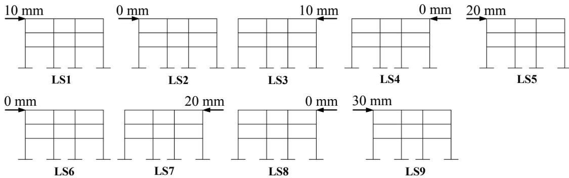
**Figure 10.** The displacement load steps applied at the RC frame
