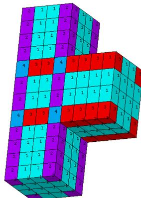
**Figure 4.** The real constant numbers at the beam-column connection
