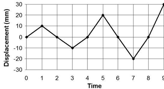
**Figure 9.** Reversed-cyclic displacement loading ( $\Delta u=10$  mm)
