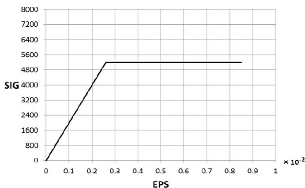
**Figure 5.** The  $\epsilon$ - $\sigma$  relationship of *Bilinear Isotropic Hardening Model* for the steel (SIG: kg/cm<sup>2</sup>)
