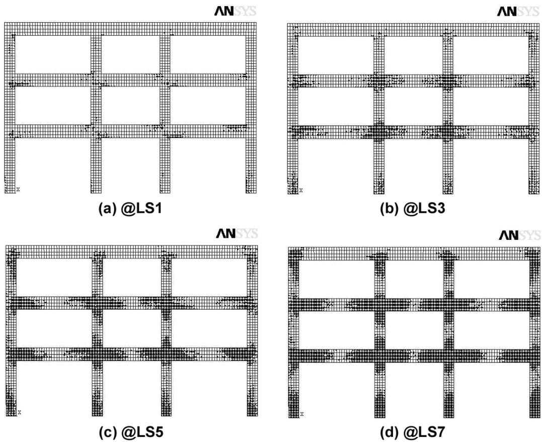
**Figure 12.** Calculated crack profiles at various load steps
