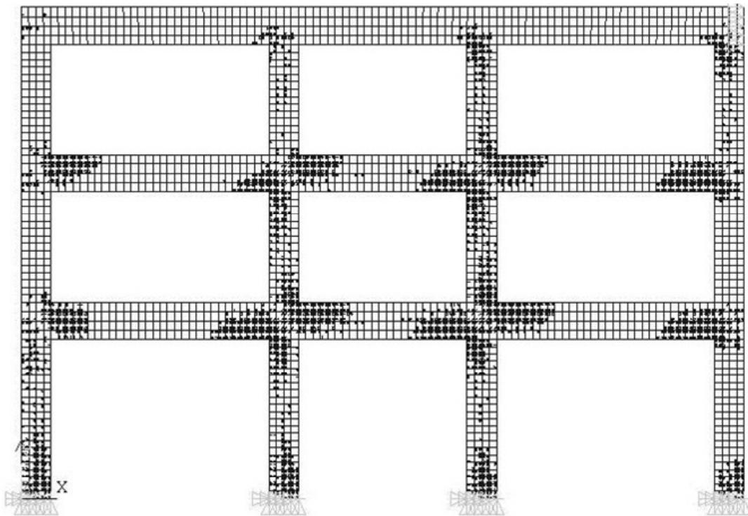
**Figure 8.** The crack profile with "third" cracks obtained from 'Analysis (a)' at maximum displacement
