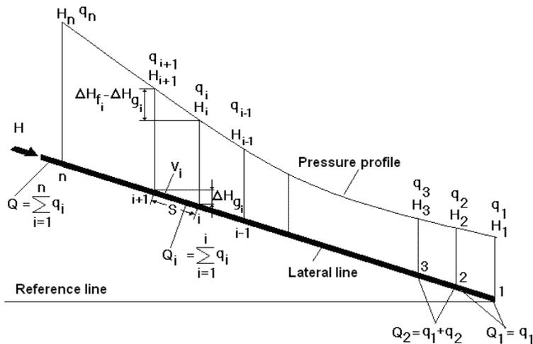
Figure 3. The pressure and flow rate distribution along the drip irrigation lateral line
