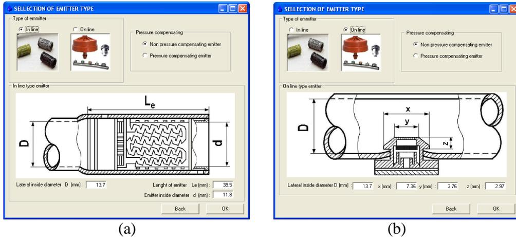
Figure 2. User interface window for selection of emitter type (a: in line) (b: on line)
