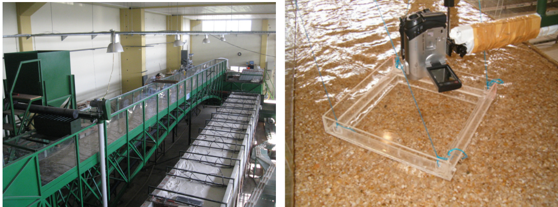
Figure 1. (a) The general view of the flume, (b) configuration of the video recorder and acrylic plate
