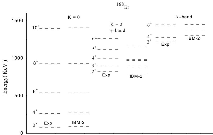
**Fig.2b.** The three lowest rotational bands in spectra of the  $^{168}\text{Er}$ . In each band the experimental data are plotted on the left and calculated values on the right
