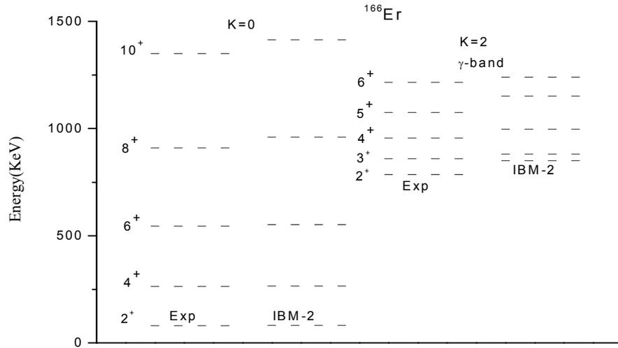
**Fig.2a** The three lowest rotational bands in spectra of the  $^{166}\text{Er}$ . In each band the experimental data are plotted on the left and calculated values on the right
