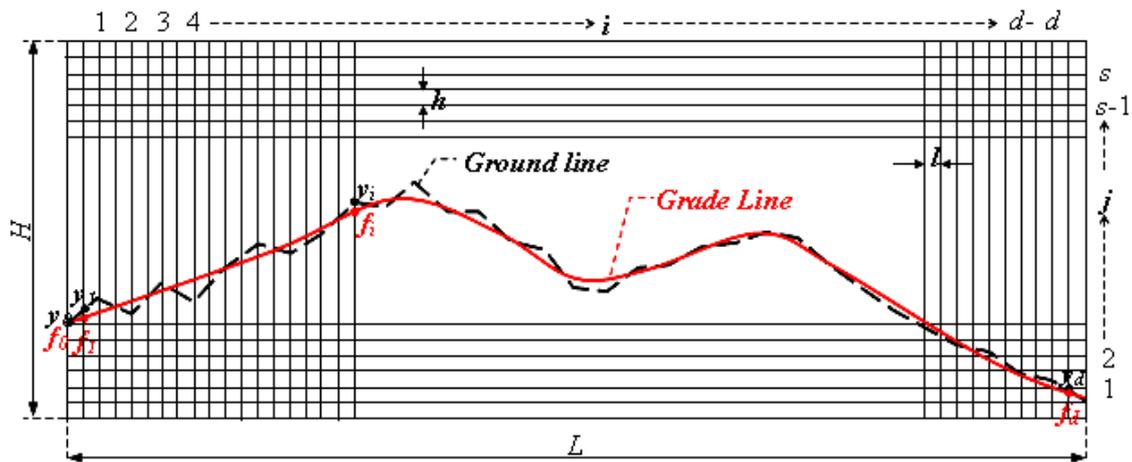
**Figure 2.** Profile for the illustration of dynamic programming model
