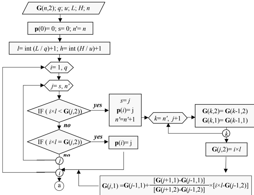
**Figure 3.** The procedure for the calculation of intersected STAs and related elevations
