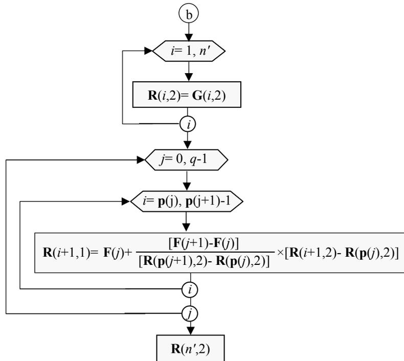
**Figure 5.** Final procedure for the calculation of final grade line matrix,  $\mathbf{R}(n,2)$
