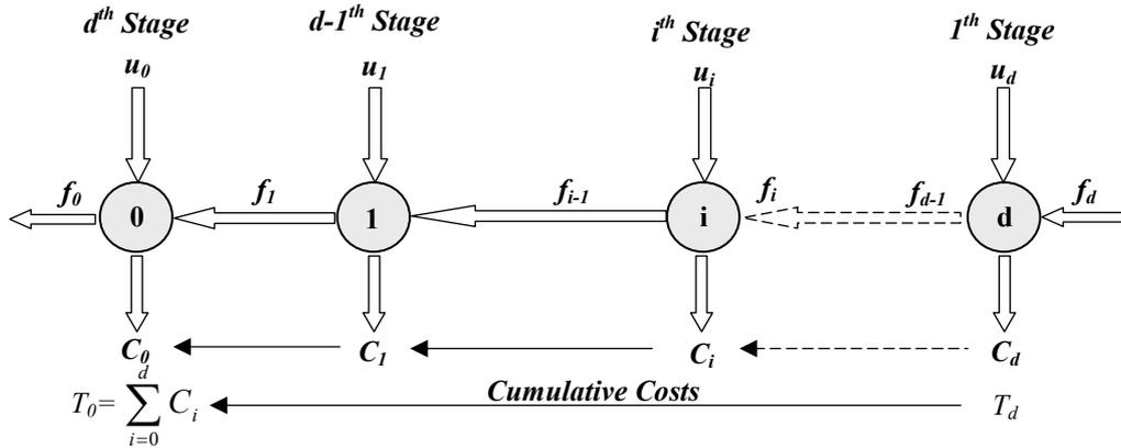
**Figure 1.** Illustration of backward dynamic programming processing scheme
