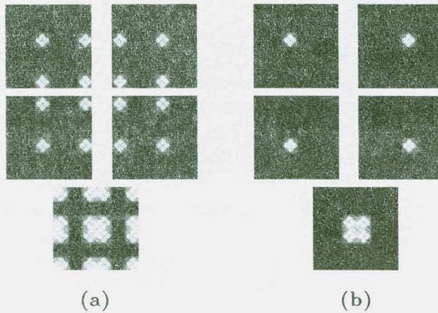
(a) Equivalent subapertures are viewed periodic and their sum before linear filtering. (b) Equivalent subapertures and their sum after linear filtering.
