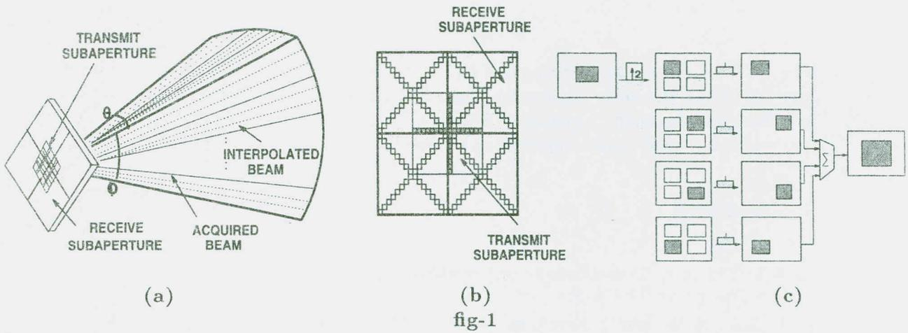
(a) Volumetric imaging. (b) Mills cross array configuration. (c) Aperture space representation of transmit and receive subapertures ( $K=2$ ) and their sum.
