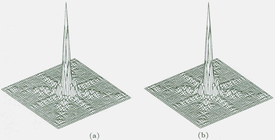
(a) Proposed technique psf and (b) Control psf. (Lateral axis:  $\sin\theta$ , Elevation axis:  $\sin\phi$ , vertical axis: amplitude.) For figure 3: ( $K = 2$ ,  $N_t^x = N_t^y = 16$ ,  $N_r^x = N_r^y = 16$ ,  $B^\theta = B^\phi = 24$ ,  $B_o^\theta = B_o^\phi = 48$ .)
