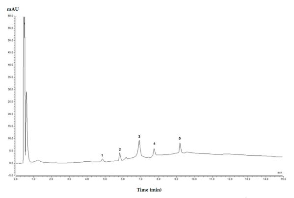
**Figure 5.** A representative chromatogram obtained from Lake water spiked at 50.0 µg·L<sup>-1</sup>, after FPSE procedure coupled with High-Performance Liquid-Chromatography–Photodiode Array Detection (FPSE-HPLC–DAD) (1. MIRT, 2. BUP, 3. CLO, 4. CIT, 5. SERT).
