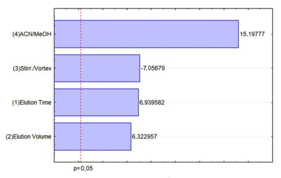
Figure 2. Pareto maps of the standardized effects (2<sup>4</sup> experimental configuration).
