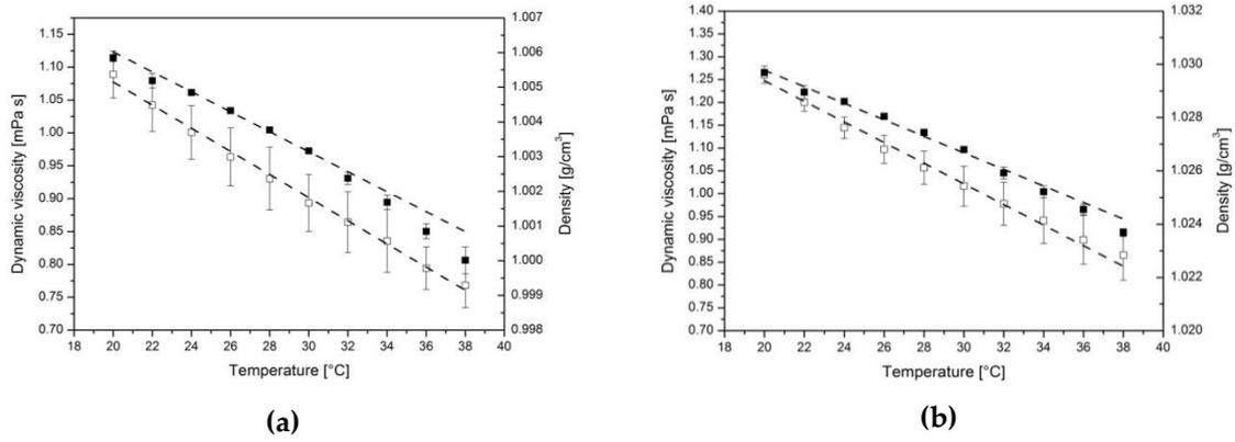
**Figure S2.** Temperature dependence of dynamic viscosity (open squares) and density (solid squares) of 20 g/kg (a) and 80 g/kg (b) sucrose solutions. The error bars correspond to the standard deviation, dashed lines represent linear fits.
