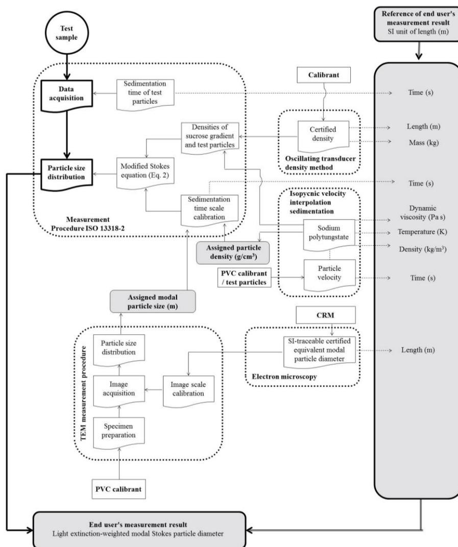
**Figure S1.** Metrological traceability network attempting to link disc-CLS particle size measurement results to the SI unit of length through PVC calibration particles characterized by transmission electron microscopy and isopycnic velocity interpolation sedimentation.
