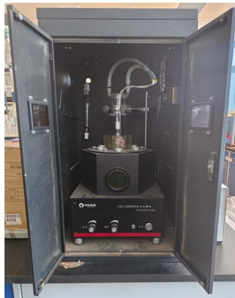
**Figure 1.** Photochemical reaction system.
