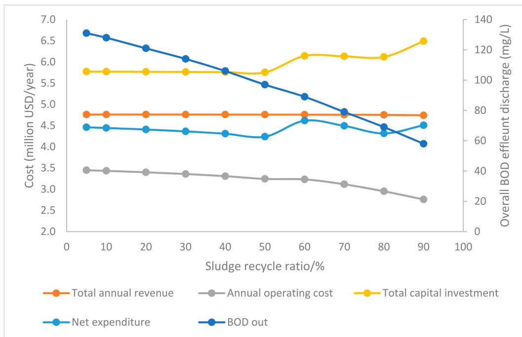
**Figure 5.** Effect of sludge recycle ratio% on economic feasibility and overall BOD effluent discharge rate.
