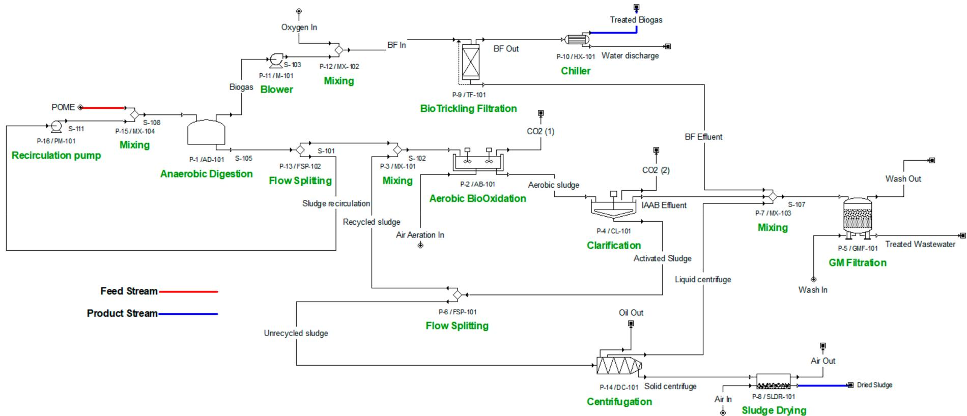
Figure 2. Process flow model for IAAB for the treatment of POME using SuperPro Designer V9.
