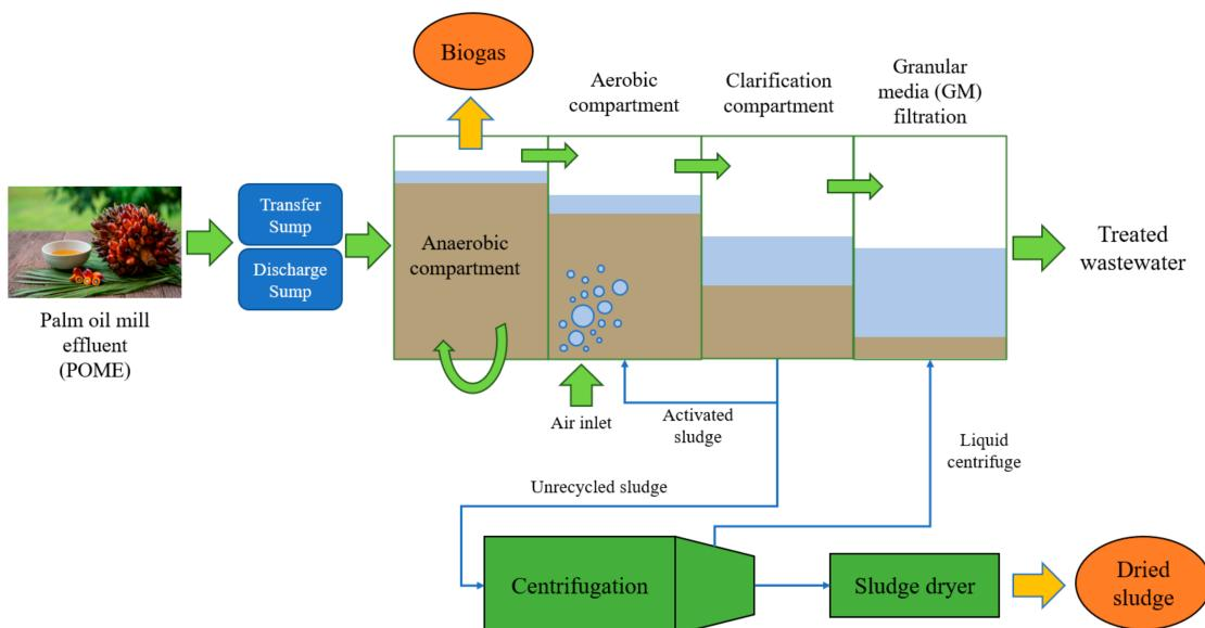
**Figure 1.** Configuration of IAAB system for the treatment of POME at industrial scale adapted from Chan et al. [18].
