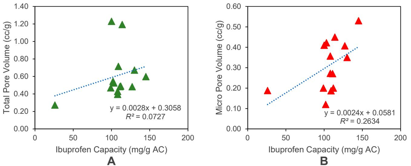
**Figure 3.** Linear regression of total pore volume (A) and micropore volume (B) of the commercial activated carbon samples and the respective ibuprofen capacities at equilibrium.
