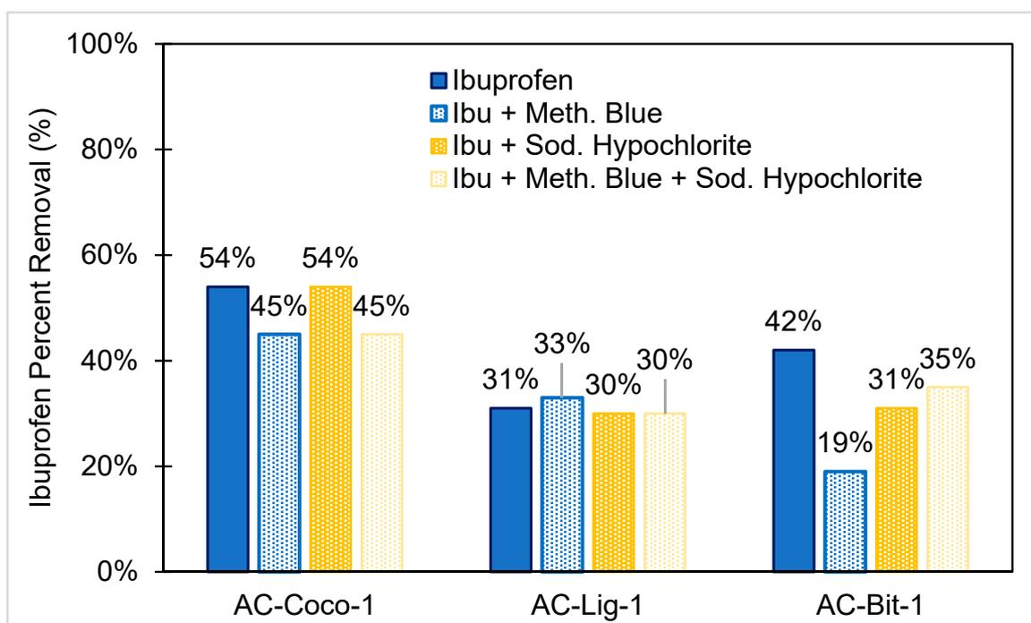
**Figure 7.** Ibuprofen removal at 1 min contact time in the presence of 3 mg/L of methylene blue and 100 mg/L sodium hypochlorite with AC-Coco-1, AC-Lig-1, and AC-Bit-1 ( $C_0 = 1.0$  g/L).
