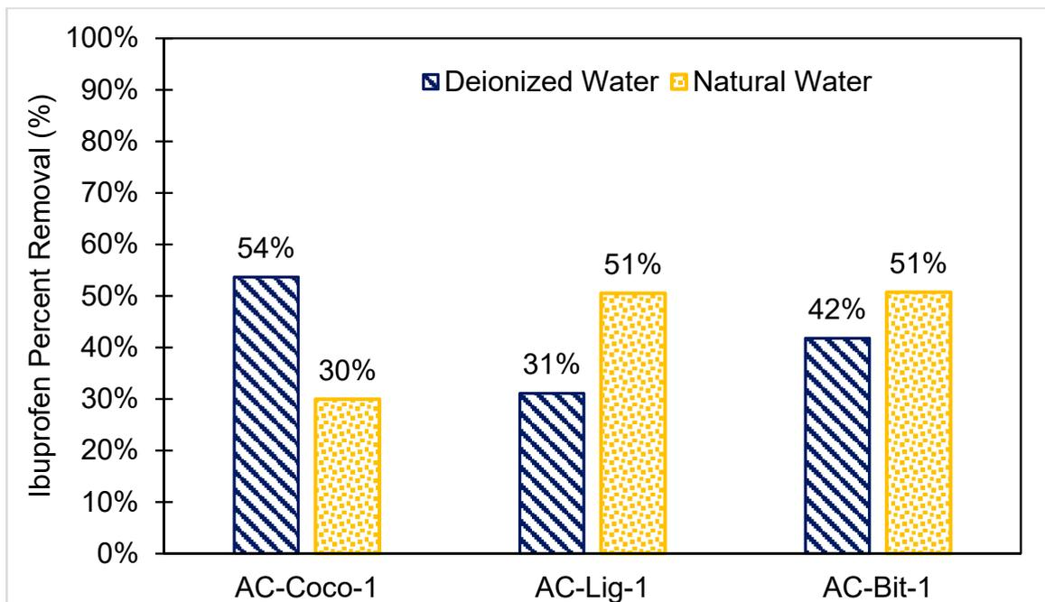
**Figure 8.** Ibuprofen adsorption at 1 min contact time of coconut, lignite, and bituminous activated carbon in deionized and natural waters ( $C_{0\text{-deionized}} = 1.0 \text{ g/L}$ ;  $C_{0\text{-natural}} = 1.1 \text{ g/L}$ ).
