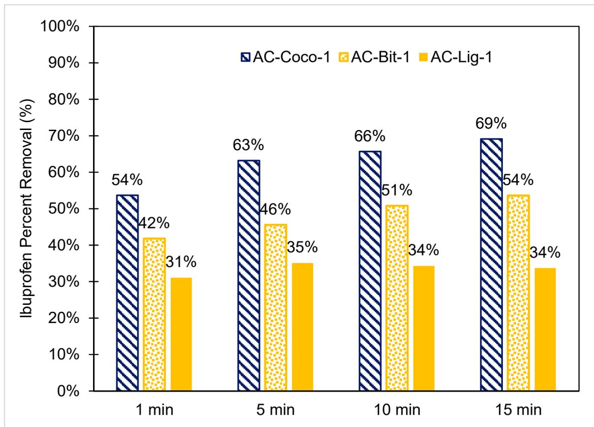
**Figure 6.** Ibuprofen kinetic removal: influence on activated carbon raw material at various contact times ( $C_0 = 1.0$  g/L).
