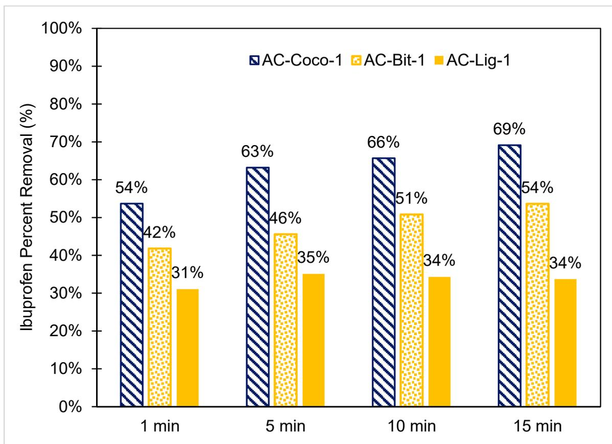
**Figure 6.** Ibuprofen kinetic removal: influence on activated carbon raw material at various contact times ( $C_0 = 1.0$  g/L).
