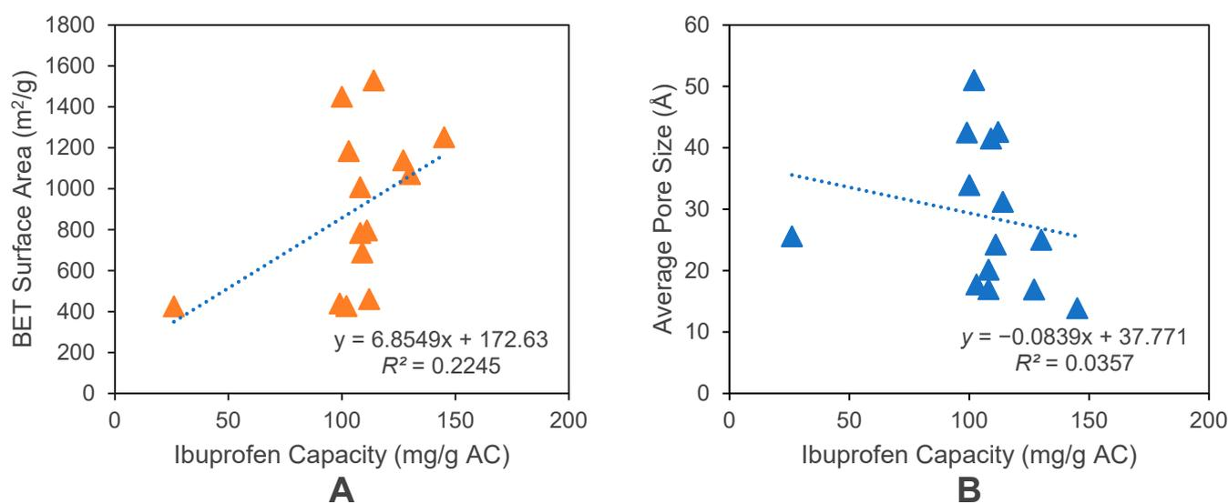
**Figure 2.** Linear regression of BET surface area (A) and average pore size (B) of the commercial activated carbon samples and the respective ibuprofen capacities at equilibrium.
