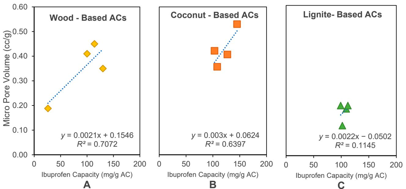
**Figure 4.** Linear regression of micropore volume vs. ibuprofen capacity at equilibrium of wood-based activated carbons (A), coconut-based activated carbons (B), and lignite-based activated carbons (C).
