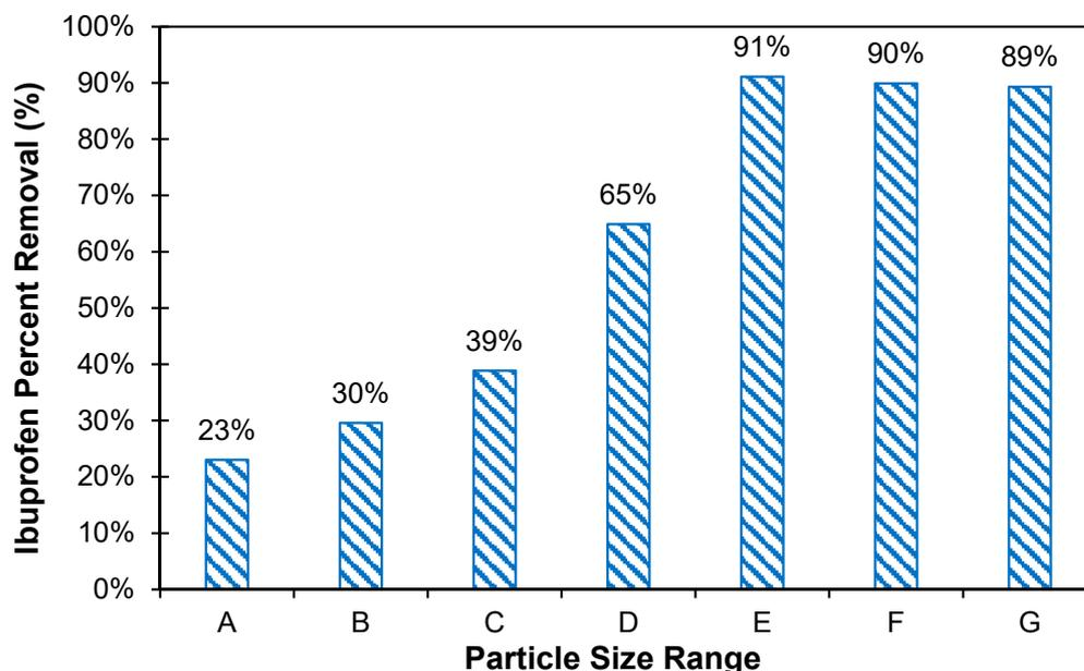
**Figure 5.** Carbon particle size distribution effect on adsorption kinetics using AC-Coco-1 (coconut) at 1 min contact time ( $C_0 = 1.0 \text{ g/L}$ ).
