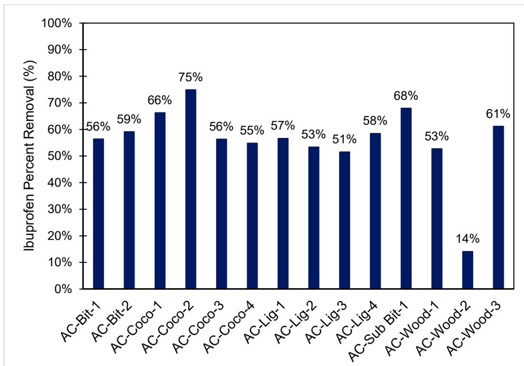
**Figure 1.** Ibuprofen removal by varying activated carbons at equilibrium (48 h) ( $C_0 = 1.0$  g/L).
