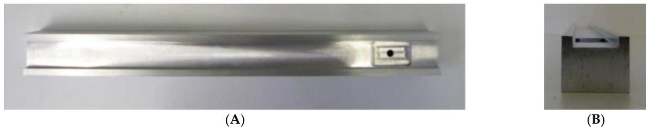
**Figure 3.** The interchangeable flow channel with a height of 5 mm: (A) top view of the flow channel and (B) side view of the flow channel.
