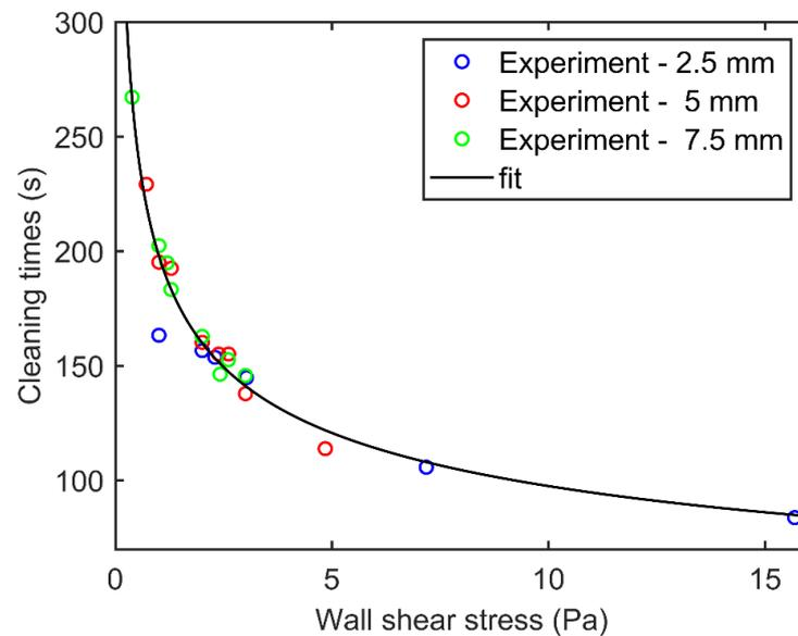
Figure 11. Cleaning times plotted against the wall shear stress.
