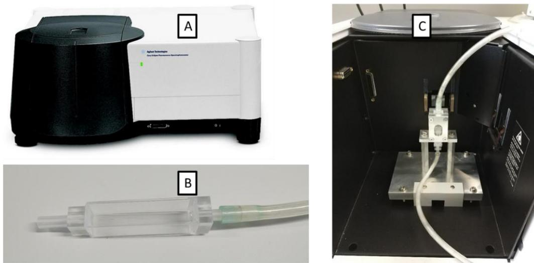
**Figure 6.** Fluorescence spectroscopy setup: (A) fluorescence spectrometer, (B) flow through cuvette, and (C) special cuvette holder.
