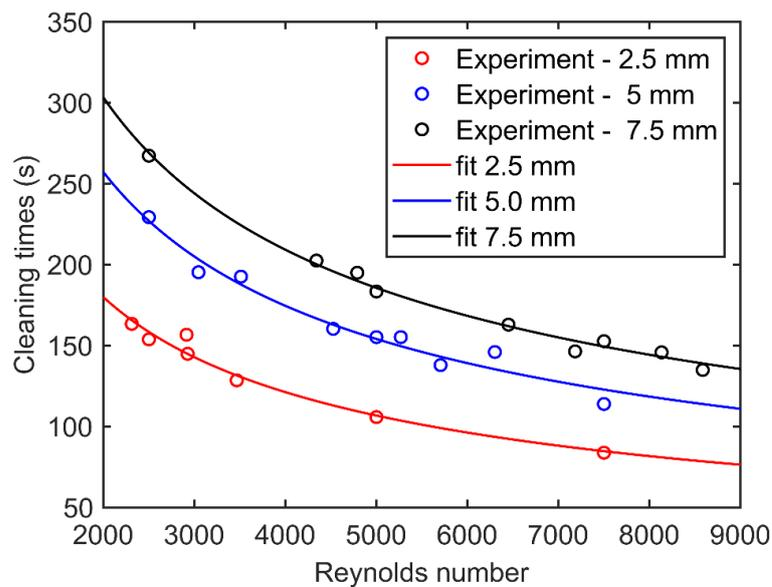
**Figure 9.** Cleaning times plotted against the Reynolds number.
