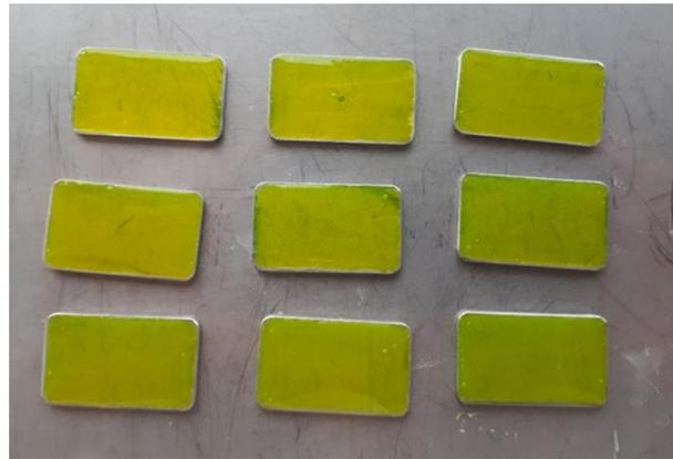
**Figure 5.** SSC samples with the fouling material.
