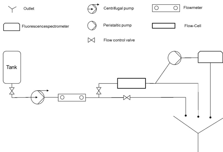
**Figure 7.** Experimental setup for cleaning tests.
