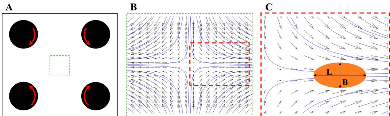
**Figure 2.** Schematically illustration of laminar breakup in a four-roller mill [33,35]: (A) The four-roller mill; (B) the laminar velocity profiles (with streamlines); (C) schematic illustration of the laminar shear experienced by a drop placed in the flow.
