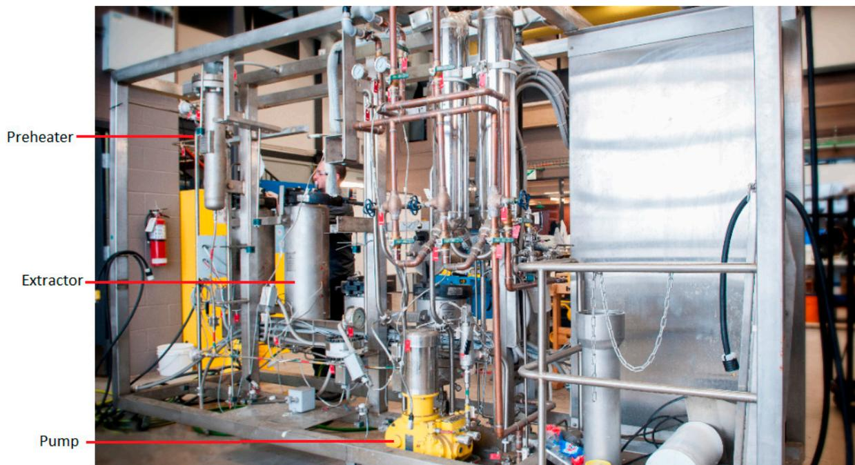
Figure 3. Experimental setup of the subcritical water extraction.
