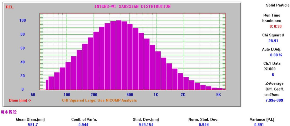
**Figure S3.** Hydrated size distribution of the polymer nanoparticle PNP.
