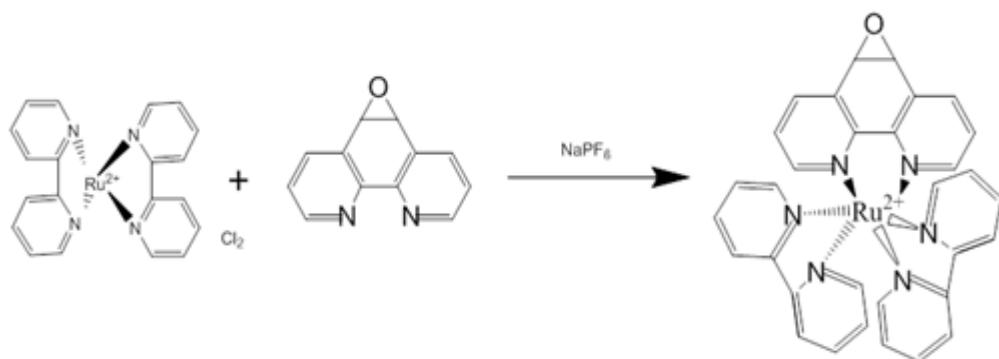
**Figure S1.** Synthesizing diagram and structure of Ru<sup>2+</sup>(bpy)<sub>2</sub>(phenepoxide).
