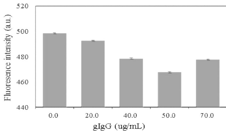
**Figure S4.** Fluorescence intensity of the supernatant after magnetic separation when adding gIgG at the concentrations of  $0 \mu\text{g mL}^{-1}$ ,  $20 \mu\text{g mL}^{-1}$ ,  $40 \mu\text{g mL}^{-1}$ ,  $50 \mu\text{g mL}^{-1}$ ,  $70 \mu\text{g mL}^{-1}$ , respectively, in the immune-reaction system.
