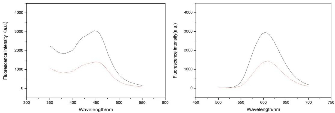
**Figure S2.** Fluorescent excitation (Upper) and emission (Lower) spectra of epo-Ru (solid line) and PAA-Ru (dash line).
