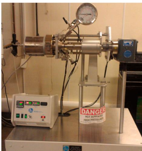
**Figure 1.** Stirred Parr reactor operating in horizontal position.
