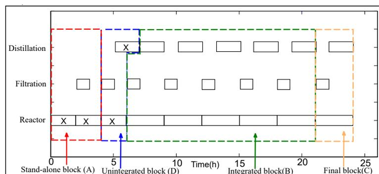
Figure 6. Optimal schedule for BR-S system for 24 h horizon.
