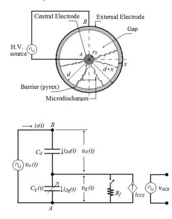
Figure 10. (a) The DBD electrode layout and (b) the equivalent circuit. Reprinted with permission from [44]. Copyright 2003, IOP Publishing.
