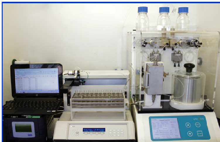
Figure 2. Continuous FlowSyn flow reactor experimental set-up.
