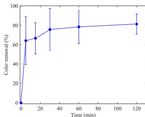
**Figure 3.** The treatment of real textile WW by the BC derived from *Pinus patula* wood pellets in terms of colour removal vs. time. Operational conditions: BC dose = 13.5 g/L, pH = 3, BC particle size = 300–450  $\mu\text{m}$ .
