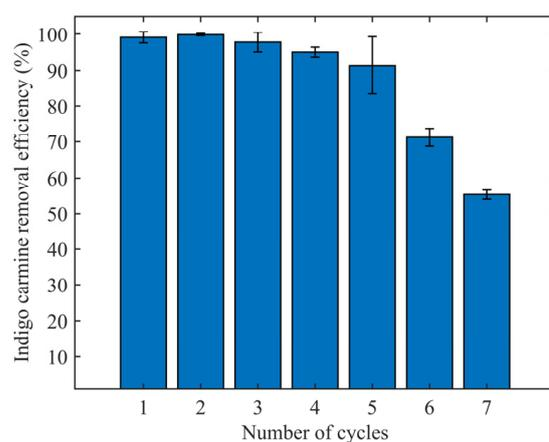
**Figure 1.** Adsorption-desorption cycles of *Pinus patula* biochar (BC). Operational conditions: BC dose = 13.5 g/L, Indigo Carmine concentration = 25 mg/L, BC particle size = 350–400  $\mu$ m, solution pH = 3, time = 5 min.
