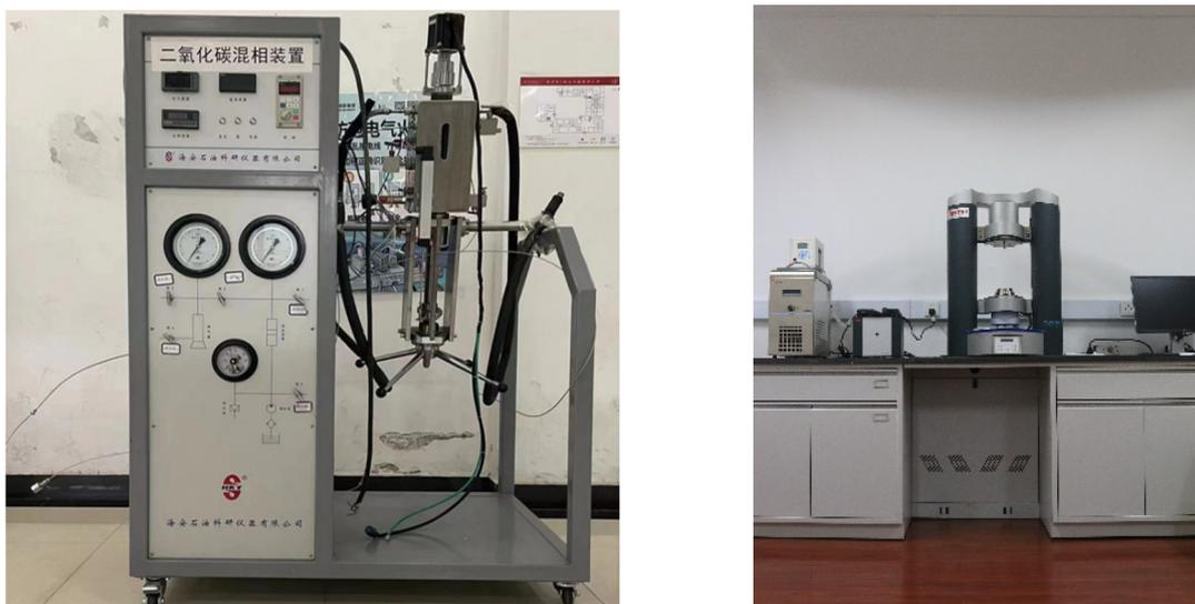
**Figure 3.** CO<sub>2</sub> fracturing fluid preparation and rheological testing device.
