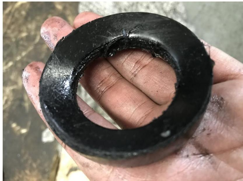
**Figure 21.** Triangular seal wear.
