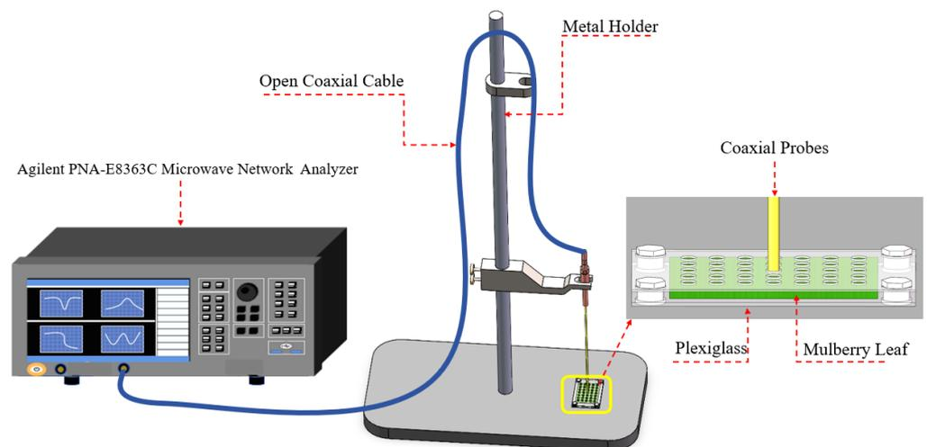
**Figure 3.** Schematic diagram of the dielectric property measurement device.
