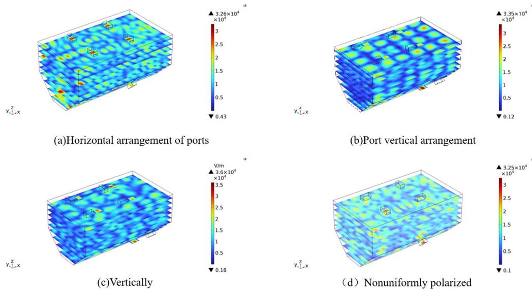
**Figure 10.** Electromagnetic field distribution in the cavity with different arrangements of ports.
