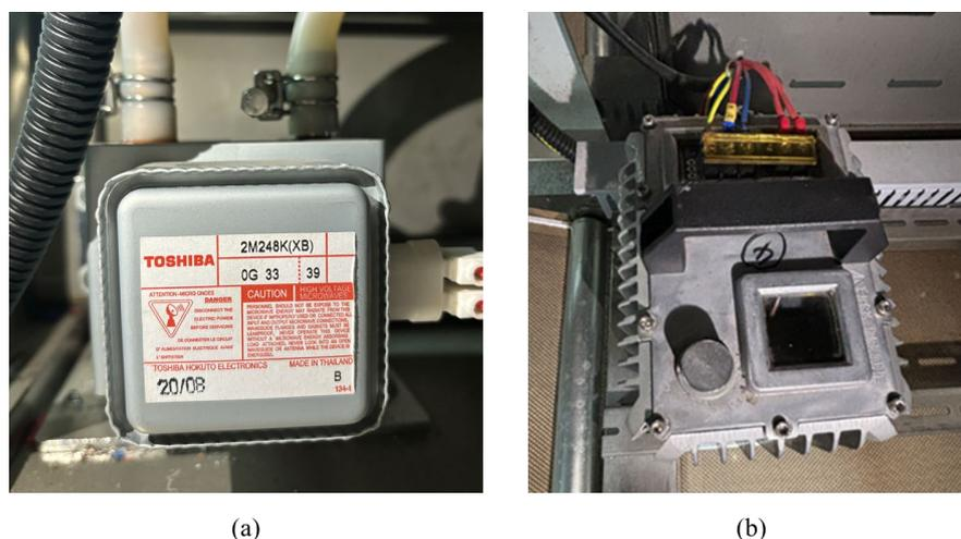
**Figure 8.** (a) Toshiba Magnetron 2M248K (XB); (b) Oil-cooled Magnetron Power Supply.
