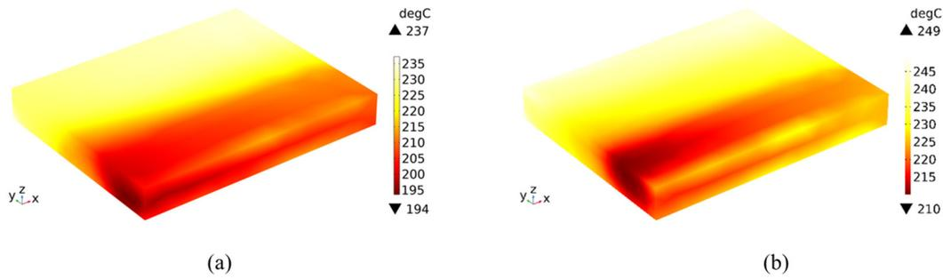
**Figure 12.** Temperature distribution of mulberry leaves under different inlet positions. (a) Temperature distribution of the first set of port parameters; (b) Temperature distribution of the seventh set of port parameters.
