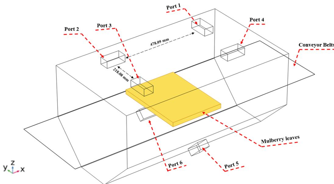
**Figure 2.** Simulation model of a continuous microwave fixation machine.
