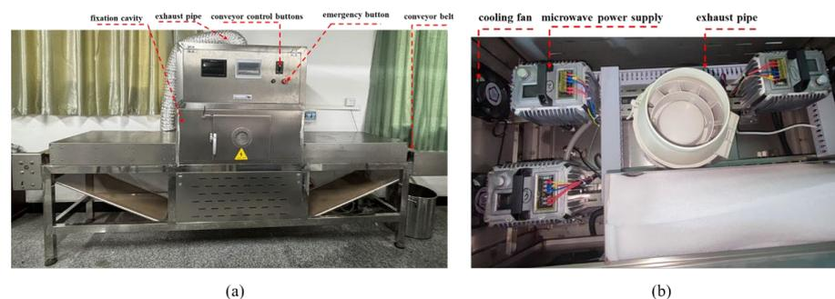
**Figure 7.** Physical system of continuous microwave fixer for mulberry leaf tea. (a) Continuous microwave mulberry leaf tea fixing machine; (b) Part of the power supply and cooling fan.
