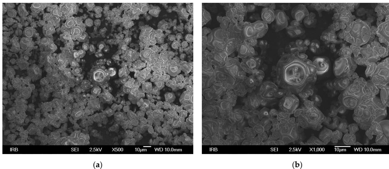
**Figure 2.** Scanning electron micrographs of the encapsulated fennel essential oil obtained under optimal spray-drying conditions (maltodextrin:gum arabic in a ratio of 1:3 spray-dried at 200 °C) with (a) 500× magnification; (b) 1000× magnification.
