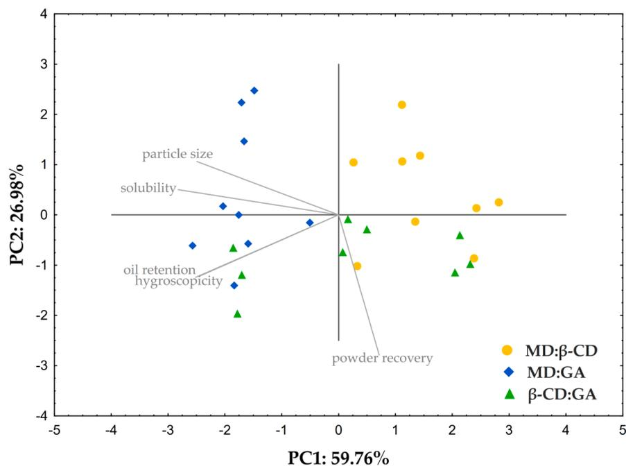
**Figure 1.** Distribution of encapsulated fennel essential oil in a two-dimensional coordinate system defined by the first two principal components (PC1 and PC2) in relation to the type of wall material.
