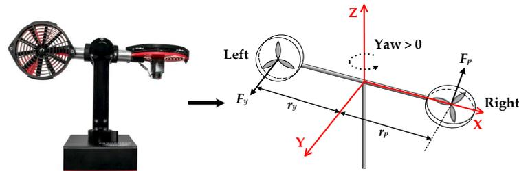
Figure 4. Half-quadrotor system and its free-body diagram.
