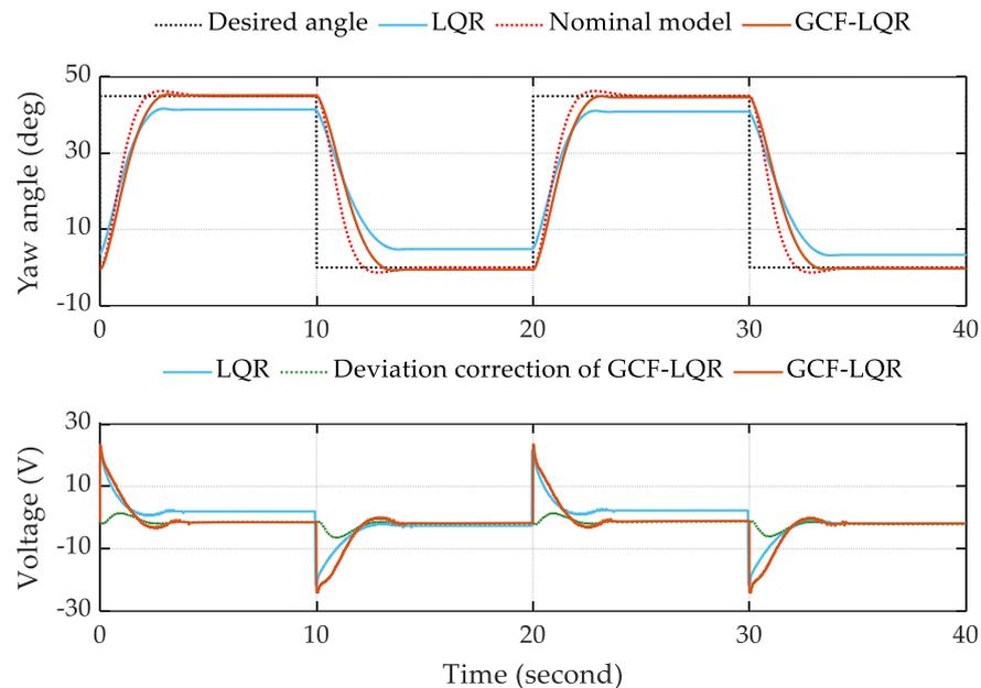
**Figure 7.** Experiment results of the standard half-quadrotor system.
