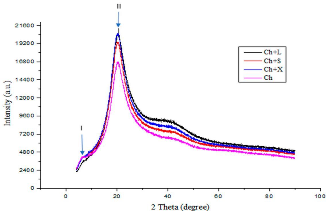
**Figure 1.** X-ray diffraction patterns of chitosan-based films enriched with 1% of *Lippia javanica* (Ch+L), *Syzygium cordatum* (Ch+S), and *Ximenia caffra* (Ch+X) extract. Ch; Chitosan. Peak I, reflection around  $2\theta = 10^\circ$ ; Peak II, reflection around  $2\theta = 20^\circ$ .
