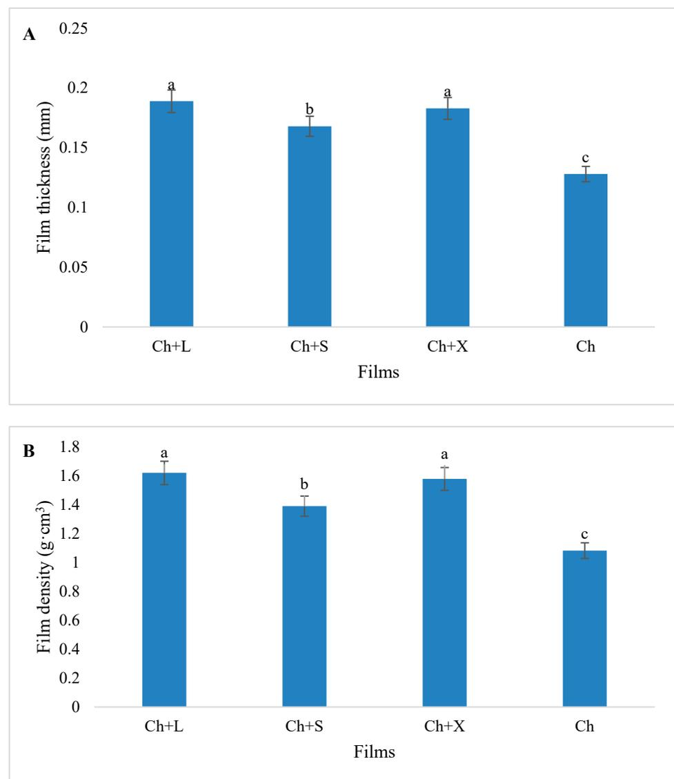
**Figure 3.** (A) Film thickness and (B) film density degree influenced by chitosan enriched with 1% of *Lippia javanica* (Ch+L), *Syzygium cordatum* (Ch+S), and *Ximenia caffra* (Ch+X) extract. Ch: chitosan only. Different letters indicate a statistical difference ( $p < 0.05$ ). Error bars denote the standard error of the mean.
