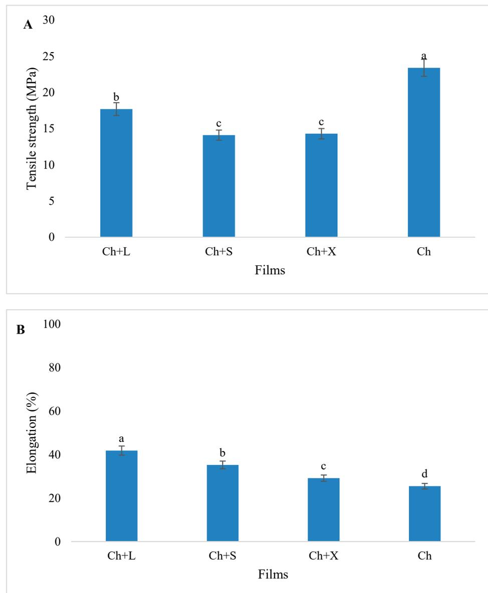
**Figure 5.** (A) Tensile strength and (B) elongation of chitosan films functionalized with 1% of *Lippia javanica* (Ch+L), *Syzygium cordatum* (Ch+S), and *Ximenia caffra* (Ch+X) extract. Ch: chitosan only. Different letters indicate a statistical difference ( $p < 0.05$ ). Error bars denote the standard error of the mean.
