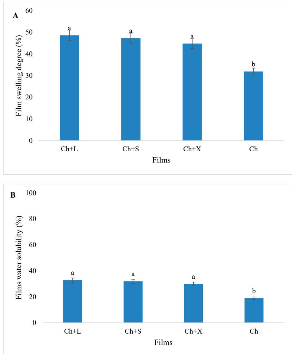
**Figure 4.** (A) Film swelling degree and (B) water solubility of chitosan films fused with 1% of *Lippia javanica* (Ch+L), *Syzygium cordatum* (Ch+S), and *Ximenia caffra* (Ch+X) extract. Ch: chitosan only. Different letters indicate a statistical difference ( $p < 0.05$ ). Error bars denote the standard error of the mean.
