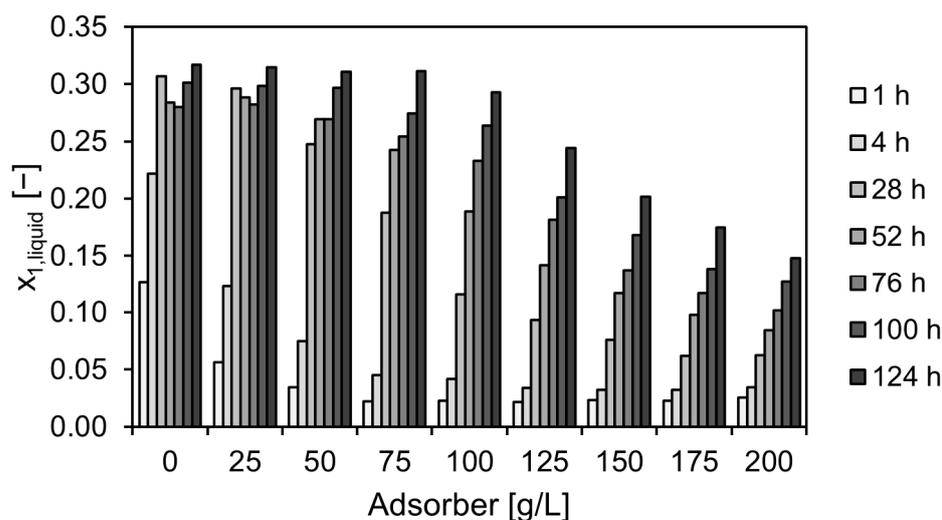
**Figure 3.** Liquid mole fraction of 2,6-DHBA in the enzymatic carboxylation of resorcinol by 0.139 g/L purified 2,6-DHBD (16.4 U/mg) in aqueous TEA saturated with CO<sub>2</sub> combined with the adsorber Dowex® 1X8-50 at 30 °C.
