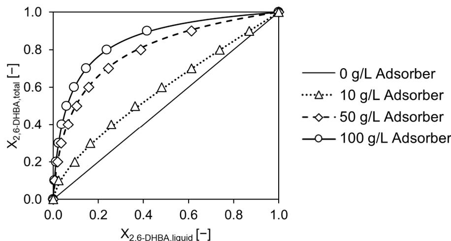
**Figure 1.** Adsorption isotherm of 80 mM mixtures of 2,6-DHBA and resorcinol on the adsorber Dowex® 1X8-50 at different concentrations in 1 M aqueous TEA saturated with CO<sub>2</sub> at 30 °C.
