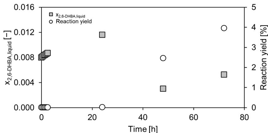
**Figure 10.** Repetitive batch of the enzymatic carboxylation of 80 mM resorcinol in 1 M aqueous TEA saturated with CO<sub>2</sub> in a 3 L stirred tank reactor with baffles. After 24 h, 30 g (20 g/L) of Dowex® 1X8-50 was added to the 1.5 L reaction medium containing 64.2 mg/L 2,6-DHBD cell-free extract. The medium was stirred at 450 rpm, heated to 30 °C and continuously gassed with 20 mL/min CO<sub>2</sub> through a 0.5 µm porous sparger.
