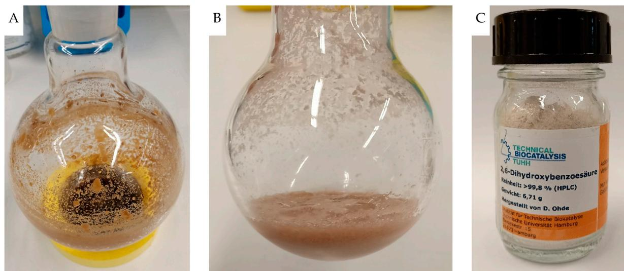
**Figure 9.** Purification status of 2,6-DHBA eluted from Dowex® 1X8-50. Following the downstream processing, (A) shows the precipitate from the elution fraction, (B) shows the 2,6-DHBA precipitate after washing with 1 M HCl and (C) shows the isolated and dried product in a glass bottle.
