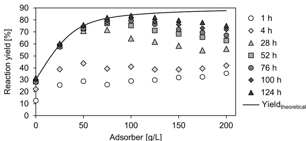
**Figure 4.** Enhancement of the enzymatic carboxylation of resorcinol by utilization of Dowex® 1X8-50. The enzymatic carboxylation of resorcinol was performed with 0.139 g/L 2,6-DHBD (16.4 U/mg) in aqueous TEA saturated with CO<sub>2</sub> at 30 °C, supplemented with Dowex® 1X8-50. The theoretical reaction yield is shown as a line, as shown in Figure 2. The reactions at high adsorber concentrations have not reached their theoretical reaction equilibrium after 124 h.
