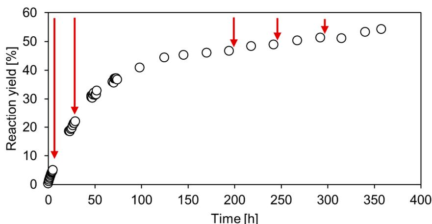
**Figure 8.** 2,6-DHBA reaction yield for the enzymatic carboxylation of 80 mM resorcinol in 1 M aqueous TEA saturated with CO<sub>2</sub> in a 3 L stirred tank reactor with baffles. In each step (indicated by red arrows), 30 g of Dowex® 1X8-50 were added to the 1.5 l reaction medium containing 64.2 mg/L 2,6-DHBD cell-free extract. The medium was stirred at 450 rpm, heated to 30 °C and continuously gassed with 20 mL/min CO<sub>2</sub> through a 0.5 µm porous sparger.
