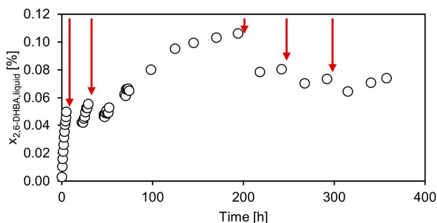
**Figure 7.** Liquid mole fraction of 2,6-DHBA during the enzymatic carboxylation of 1.5 L of 80 mM resorcinol in 1 M aqueous TEA saturated with CO<sub>2</sub> in a 3 L stirred tank reactor with baffles. In each step (indicated by red arrows), 30 g of Dowex® 1X8-50 were added to the 1.5 L reaction medium containing 64.2 mg/L 2,6-DHBD cell-free extract. The medium was stirred at 450 rpm, heated to 30 °C and continuously gassed with 20 mL/min CO<sub>2</sub> through a 0.5 µm porous sparger.
