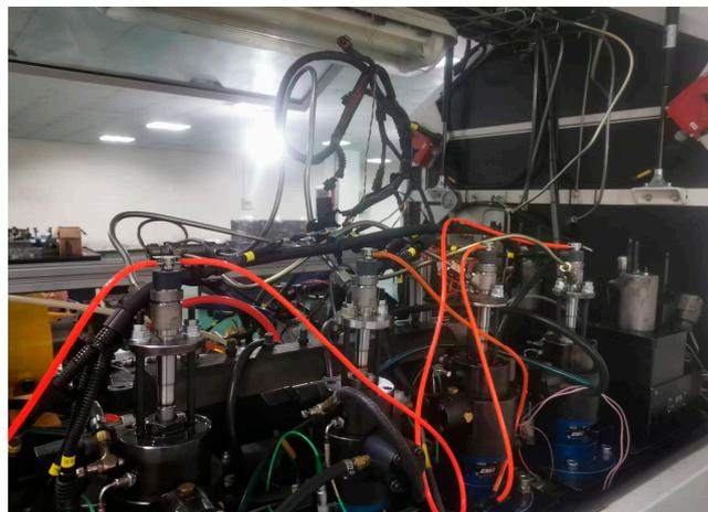
**Figure 19.** Test platform of the HPCRIS for diesel engines.
