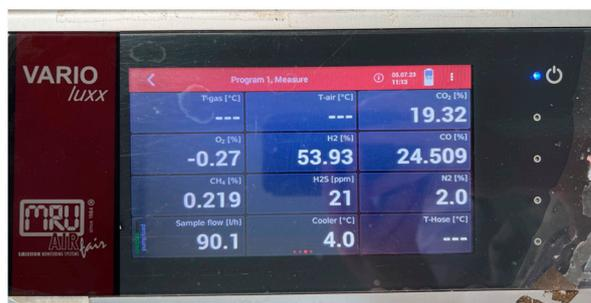
Figure 2. Gas analyzer (MRU model, Vario luxx).
