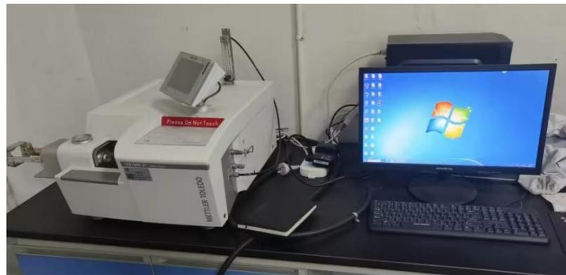
**Figure 1.** Mettler Toledo TGA/DSC3<sup>+</sup> synchronous thermal analyzer.
